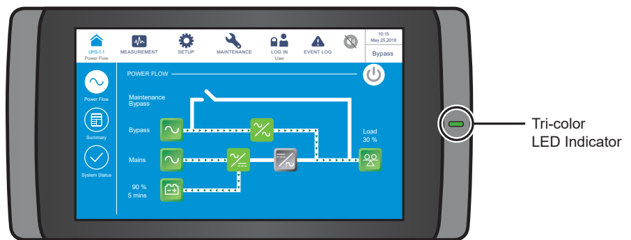
(Figure 2-11: Tri-color LED Indicator Location)
