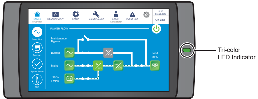
(Figure 2-11: Tri-color LED Indicator Location)
