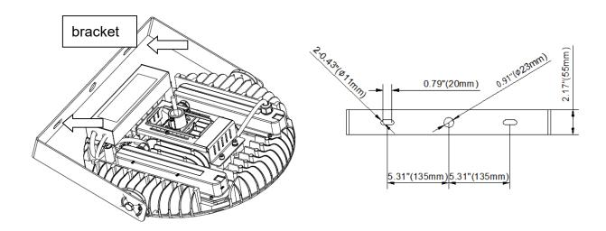
2. Loosen the M10 and M4 screw, and tilt the luminaire to the determined direction. If determined, fixed the Screw.
