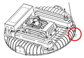
2.Attach other end of the safety cable to the mounting surfaces.
