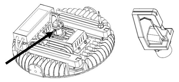
2. The Weight of High Bay fixture is approximately 19.8 lb(9 Kg). Please ensure the structure and the suspending cable/chain are suitable for the weight of the fixture.
