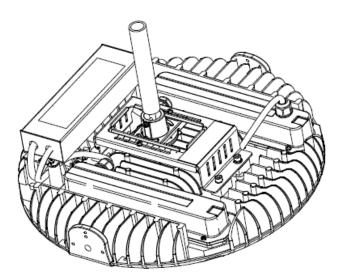
2. Insert set screw in order to secure the fixture to the Pipe to prevent loosening.
