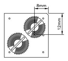
**Figure 5:** Temperature measurement location
