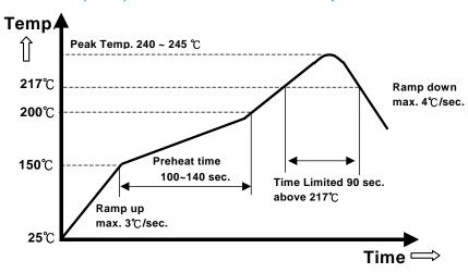
Note: The temperature refers to the pin of filter 7A, measured on the pin 1 (+Vout) joint.
