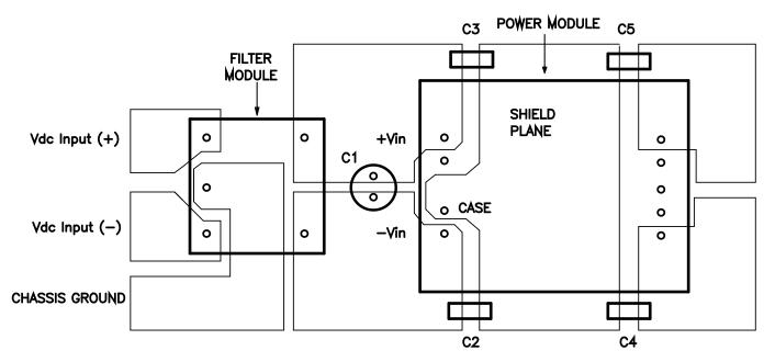
Note: Avoid routing signals or planes under the power module or the filter module. Please ensure all connections are low impedance.
