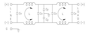
Figure 3: Internal schematics
