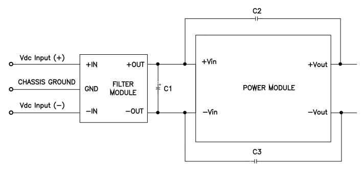
Note: C2 & C3 can be  $0.01\mu\text{F}$  to  $0.1\mu\text{F}$ . Select the voltage rating to meet input-to-output isolation requirements. C1 should be the recommended value suggested in the power module data sheet.
