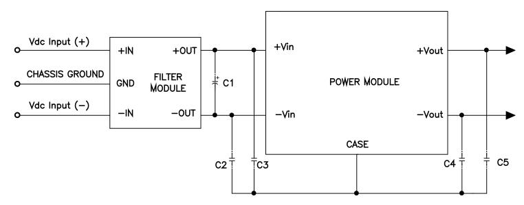
Note: C2 through C5 can be  $0.01\mu\text{F}$  to  $0.1\mu\text{F}$ . Select the voltage rating to meet input-to-output isolation requirements. C1 should be the recommended value suggested in the power module data sheet.
