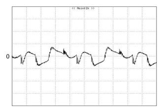
Figure 13: Output voltage ripple at nominal input voltage and rated load current (50 mV/div, 1us/div)
