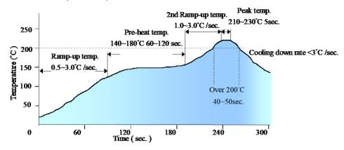
Note: The temperature refers to the pin of V48SH, measured on the pin +Vout joint.
