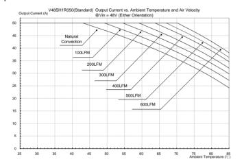
**Figure 20:** Output current vs. ambient temperature and air velocity @Vin=48V(Either Orientation, airflow from Vin+ to Vout+, without heat spreader)
