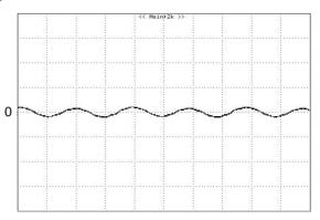
**Figure 10:** Input Terminal Ripple Current, i<sub>c</sub>, at full rated output current and nominal input voltage with 12μH source impedance and 33μF electrolytic capacitor (200 mA/div, 1us/div)
