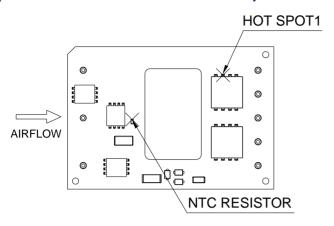
Figure 19: \* Hot spot 1& NTC resistor temperature measured points
