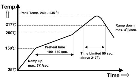
Note: The temperature refers to the pin of V48SH, measured on the pin +Vout joint.
