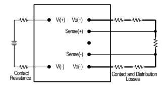
**Figure 15:** Effective circuit configuration for remote sense operation
