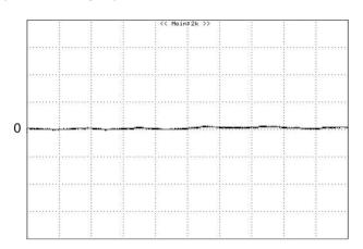
**Figure 11:** Input reflected ripple current, is, through a 12µH source inductor at nominal input voltage and rated load current (20 mA/div, 1us/div)
