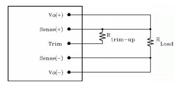
Figure 17: Circuit configuration for trim-up (increase output voltage)
