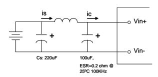
**Figure 9:** Test set-up diagram showing measurement points for Input Terminal Ripple Current and Input Reflected Ripple Current.
