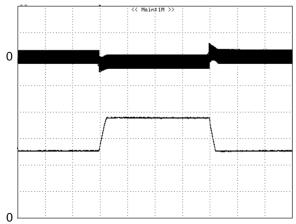
**Figure 8:** Output voltage response to step-change in load current (75%-50%-75% of Io, max; di/dt = 0.1A/ $\mu$ s). Load cap: 10 $\mu$ F tantalum capacitor and 1 $\mu$ F ceramic capacitor. Top Trace: Vout (50mV/div, 500us/div), Bottom Trace: lout (10A/div). Scope measurement should be made using a BNC cable (length shorter than 20 inches). Position the load between 51 mm to 76 mm (2 inches to 3 inches) from the module
