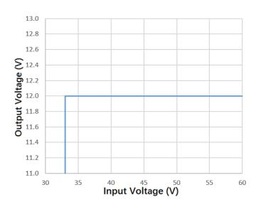
Figure 4: Input Voltage vs. Output Voltage
