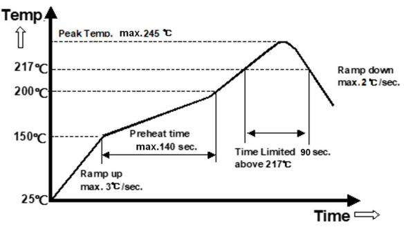
Suggested Temperature Profile for Lead-free Reflow Soldering Note: The temperature is measured on solder joint of pins of power module
