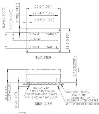
NULES: DIMENSIONS ARE IN MILLIMETERS AND (INCHES) TOLERANCES: X.Xmm±0.5mm(X.XX in.±0.02 in.) X.XXmm±0.25mm(X.XXX in.±0.010 in.)
