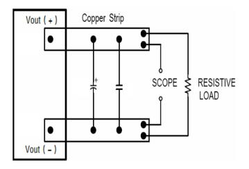
Figure 11: Test Setup for Output Voltage Noise and Ripple
