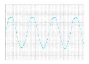
Figure 10: Input Terminal Ripple Current, i<sub>c</sub>, at max output current and nominal input voltage with  $12\mu$ H source impedance and  $100\mu$ F electrolytic capacitor (1A/div, 2us/div).
