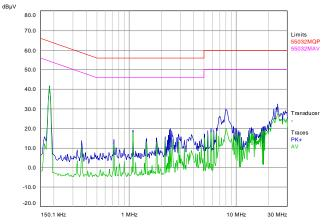
Figure 13-2: Test Result of EMC (Vin=54V, full load).
