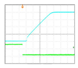
Figure 5: Remote On/Off (negative logic) at full load Vin=54V,  $I_{out} = I_{o, max}$ Time: 4ms/div. V<sub>out</sub> (top trace): 3V/div; V<sub>remote On/Off signal</sub> (bottom trace): 1V/div.
