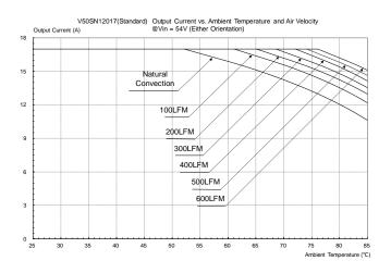
**Figure 18:** Output Power vs. Ambient Temperature and Air Velocity @Vin = 54V (Either Orientation, Open Frame)
