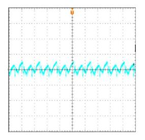
**Figure 12: Output Voltage Ripple and Noise** at nominal input voltage and max load current (30mV/div, 4us/div) Load cap: 580uF, 110uF Ceramic Capacitor,470uF Oscon cap.
