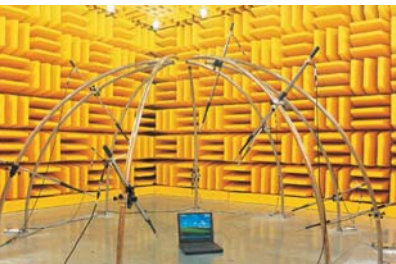
Anechoic Chamber for Noise Test
