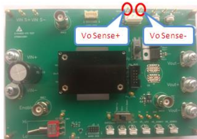
Fig-4 Vout test point
