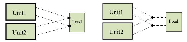
Figure 11: suggested parallel connections
