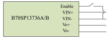
Figure 10: suggested Enable connection
