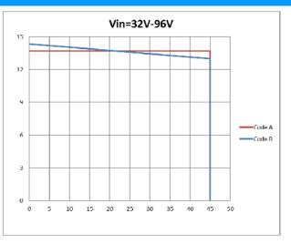
**Figure 8:** Output voltage vs. Output current OCL Performance
