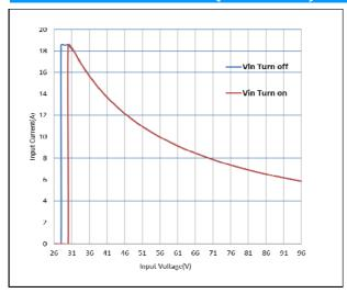
**Figure 7:** Input current vs. Input voltage @Full load
