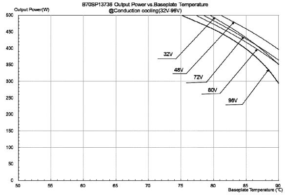
Figure 14: Output Power vs. baseplate temperature
