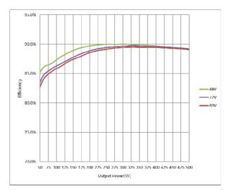
**Figure 1:** Efficiency vs. Output Power @ Vin=48V,72V,80V
