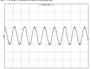
Figure 5: Output ripple & noise at 72Vin, 100% lout CH1:VOUT, 100mV/div, 5uS/div
