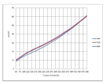
Figure 2: Loss vs. Output Power @ Vin=48V,72V,80V
