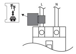
(3) Connect the current sensor cable to the current sensor connection terminal of the measurement unit.
