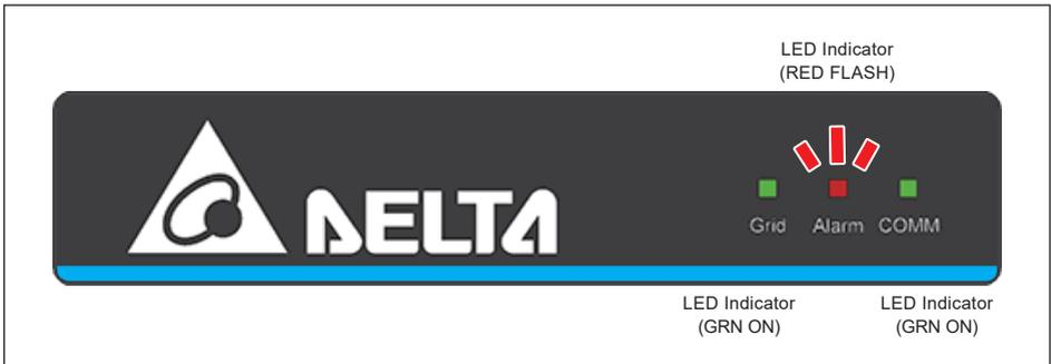
**Figure 5-5: Display Indicating AC and DC SPD failure**
