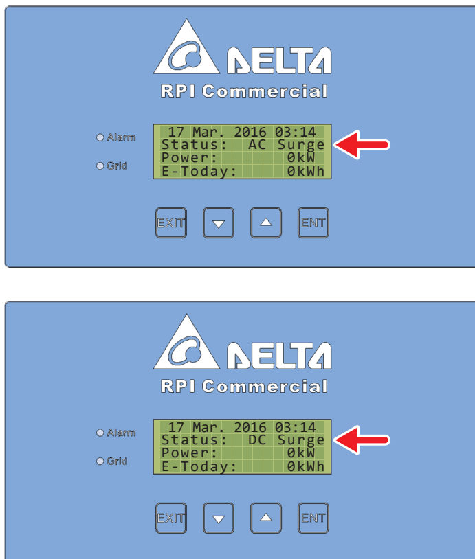
Figure 5-4: Display Indicating AC and DC SPD failure
