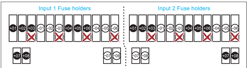
Figure 3-17: Prohibited fuse location using 20A fuse
