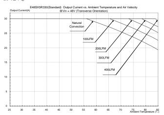
Thermal Curves (With Heat-Spreader)
