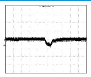
**Figure 9:** Output voltage response to step-change in load current (50%-75% of Io, max; di/dt =  $0.1A/\mu s$ ). Load cap:  $10\mu F$ , tantalum capacitor and  $1\mu F$  ceramic capacitor. Trace: Vout (50mV/div, 100us/div), Scope measurement should be made using a BNC cable (length shorter than 20 inches). Position the load between 51 mm to 76 mm (2 inches to 3 inches) from the module.
