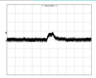
**Figure 8:** Output voltage response to step-change in load current (75%-50% of Io, max; di/dt =  $0.1A/\mu s$ ). Load cap:  $10\mu F$ , tantalum capacitor and  $1\mu F$  ceramic capacitor. Trace: Vout (50mV/div, 100us/div), Scope measurement should be made using a BNC cable (length shorter than 20 inches). Position the load between 51 mm to 76 mm (2 inches to 3 inches) from the module.
