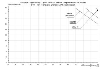
Figure 22: Output current vs. ambient temperature and air velocity Figure 24: Output current vs. ambient temperature and air velocity Vin+, without heat spreader) Vin+, with heat spreader)
