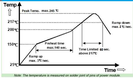
The module's top side Q2/Q4/Q101/Q102/Q103/Q104/Q508/L2 that under heat-spreader are critical components, customer must make sure these components solder joint temperature below 210°C when customer reflow solder the model to customer system board.
