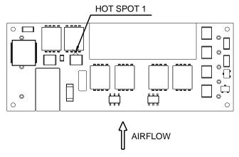
Figure 21: \* Hot spot 1& NTC resistor temperature measured points. The allowed maximum hot spot 1 temperature is defined at 124°C
