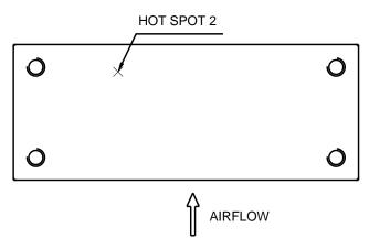
Figure 23: \* Hot spot 2 temperature measured point. The allowed maximum hot spot 2 temperature is defined at 114°C
