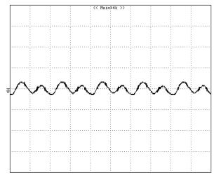
**Figure 11:** Input Terminal Ripple Current, ic, at full rated output current and nominal input voltage with 12μH source impedance and 33μF electrolytic capacitor (200 mA/div, 2us/div).
