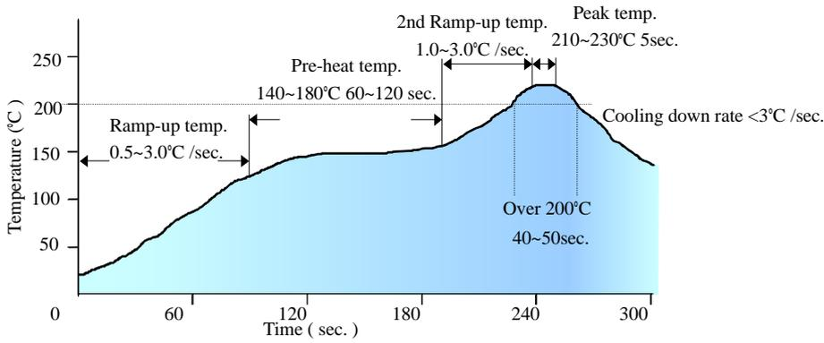
Note: The temperature refers to the pin of E48SP, measured on the pin +Vout joint.
