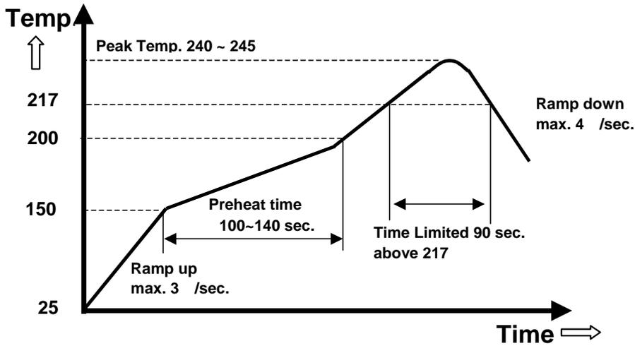
Note: The temperature refers to the pin of E48SP, measured on the pin +Vout joint.
