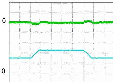
**Figure 8:** Output voltage response to step-change in load current (75%-50%-75% of  $I_{o, max}$ ;  $di/dt = 0.1A/\mu s$ ). Load cap: 10 $\mu F$  tantalum capacitor and 1 $\mu F$  ceramic capacitor. Top Trace:  $V_{out}$  (100mV/div, 200us/div), Bottom Trace:  $I_{out}$  (20A/div). Scope measurement should be made using a BNC cable (length shorter than 20 inches). Position the load between 51 mm to 76 mm (2 inches to 3 inches) from the module
