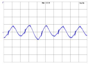
*Figure 24:* Output voltage ripple at Vin=72V and full load Trace: Vout, 100 mV/div, 2us/div; Bandwidth: 20 MHz.
