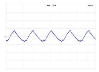
**Figure 12:** Output voltage ripple at Vin=72V and full load Trace: Vout, 100mV/div, 2us/div; Bandwidth: 20 MHz.
