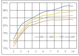
Figure 13: Efficiency vs. load current at 25°C.
