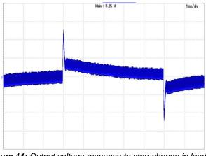
**Figure 11:** Output voltage response to step-change in load current (50%-75%-50% of full load; di/dt = 0.1A/µs). Trace: Vout, 200mV/div; Time: 1ms/div
