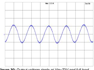
*Figure 30:* Output voltage ripple at Vin=72V and full load Trace: Vout, 100 mV/div, 2us/div; Bandwidth: 20 MHz.
