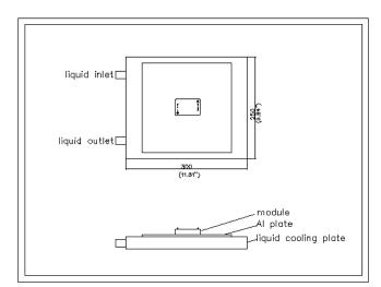
Figure 32: Thermal Test setup
