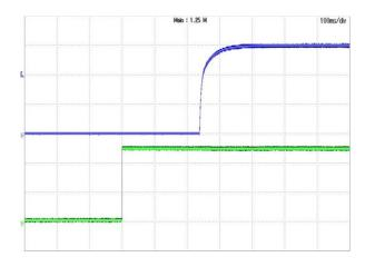
**Figure 16:** Turn-on transient at full load current (100ms/div). Top Trace: Vout, 5V/div; Bottom Trace: ON/OFF, 5V/div
