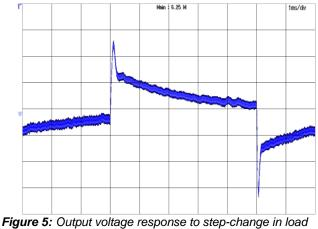
**Figure 5:** Output voltage response to step-change in load current (50%-75%-50% of full load; di/dt = 0.1A/µs). Trace: Vout, 100mV/div; Time: 1ms/div
