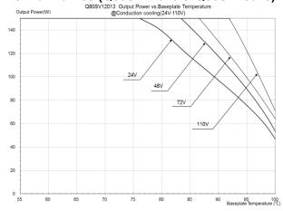
Figure 35: Output power vs. base plate temperature  $@V_{in}=24$ ~110V  $V_{out}=12V$  or 15V
