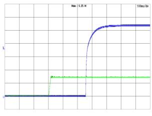
Figure 27: Turn-on transient at full load current (100ms/div).
