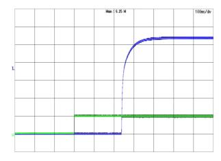
*Figure 28:* Turn-on transient at full load current (100ms/div). Top Trace: Vout, 10V/div; Bottom Trace: ON/OFF, 5V/div
