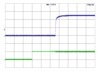
*Figure 4:* Turn-on transient at full load current (100ms/div). Top Trace: Vout, 2V/div; Bottom Trace: ON/OFF, 5V/div
