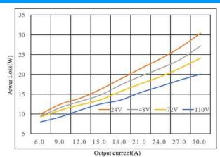
Figure 2: Power loss vs. load current at 25°C.
