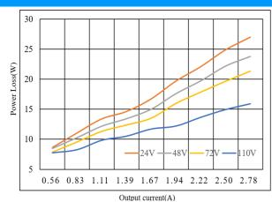
Figure 26: Power loss vs. load current at 25°C.
