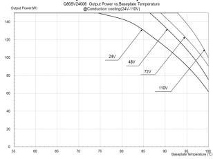
Figure 36: Output power vs. base plate temperature  $@V_{in}=24$ ~110V  $V_{out}=24V$
