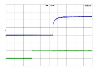
*Figure 22:* Turn-on transient at full load current (100ms/div). Top Trace: Vout, 5V/div; Bottom Trace: ON/OFF, 5V/div
