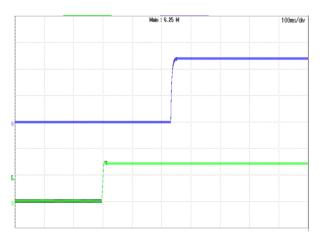
*Figure 9:* Turn-on transient at full load current (100ms/div). Top Trace: Vout, 5V/div; Bottom Trace: Vin, 50V/div
