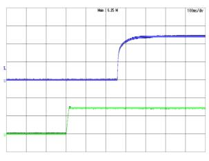
*Figure 21:* Turn-on transient at full load current (100ms/div). Top Trace: Vout, 5V/div; Bottom Trace: Vin, 50V/div
