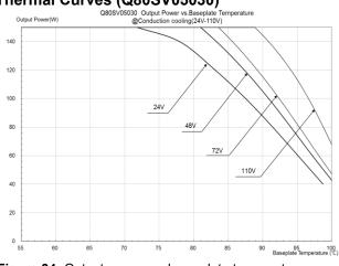
Figure 34: Output power vs. base plate temperature  $@V_{in}=24$ ~110V  $V_{out}=5V$
