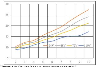
Figure 14: Power loss vs. load current at 25°C.
