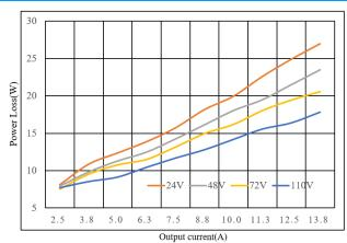
Figure 8: Power loss vs. load current at 25°C.
