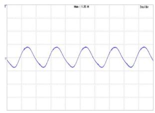
*Figure 18:* Output voltage ripple at Vin=72V and full load Trace: Vout, 100 mV/div, 2us/div; Bandwidth: 20 MHz.
