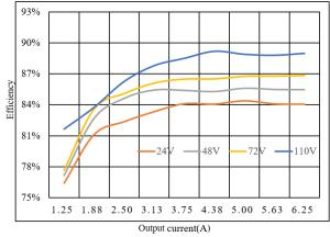
Figure 19: Efficiency vs. load current at 25°C.
