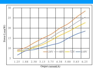
Figure 20: Power loss vs. load current at 25°C.
