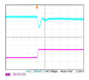
**Figure 8:** Output voltage response to step-change in load current (25%-75% of Io, max; di/dt = 1A/μs; Vin=48V). Load cap: 1mF tantalum capacitor and 1μF ceramic capacitor. Top Trace: Vout (0.2V/div, 100us/div), Bottom Trace: lout (20A/div). Scope measurement should be made using a BNC cable (length shorter than 20 inches). Position the load between 51 mm to 76 mm (2 inches to 3 inches) from the module
