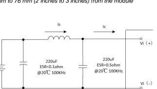
**Figure 10:** Test set-up diagram showing measurement points for Input Terminal Ripple Current and Input Reflected Ripple Current.
