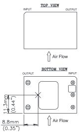
Figure 18: \* Hot spot 1's temperature measured point. Figure 20: \* Hot spot 2's temperature measured point. The allowed maximum hot spot's temperature is defined at 120  $\mathcal{C}$ . The allowed maximum hot spot's temperature is defined at 120  $\mathcal{C}$ .
