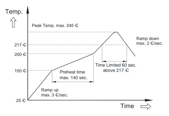
Recommended Temperature Profile for Lead-free Reflow Soldering Note: The temperature is measured on solder joint of pins of power module.
