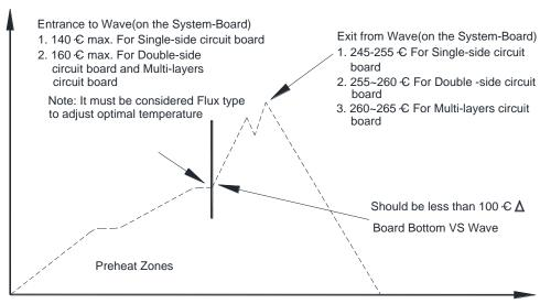
Recommended Temperature Profile for Lead-free Wave Soldering Note: The temperature is measured on solder joint of pins of power module.
