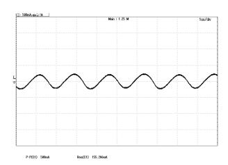
**Figure 11:** Input Terminal Ripple Current, i<sub>c</sub>, at max output current and nominal input voltage with 12μH source impedance and 220μF electrolytic capacitor (500 mA/div, 1us/div).
