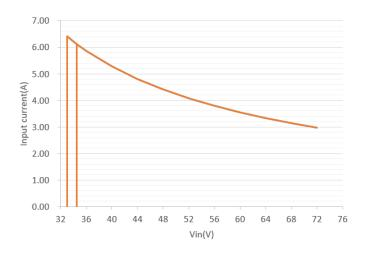
Figure 3: Full load input characteristics at room temperature.
