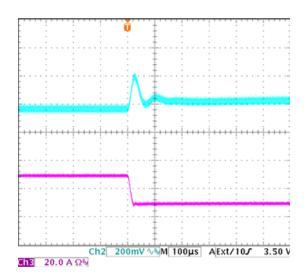
**Figure 9:** Output voltage response to step-change in load current (75%-25% of lo, max; di/dt = 1A/μs; Vin=48V). Load cap: 1mF tantalum capacitor and 1μF ceramic capacitor. Top Trace: Vout (0.2 V/div, 200us/div), Bottom Trace: lout (20A/div). Scope measurement should be made using a BNC cable (length shorter than 20 inches). Position the load between 51 mm to 76 mm (2 inches to 3 inches) from the module
