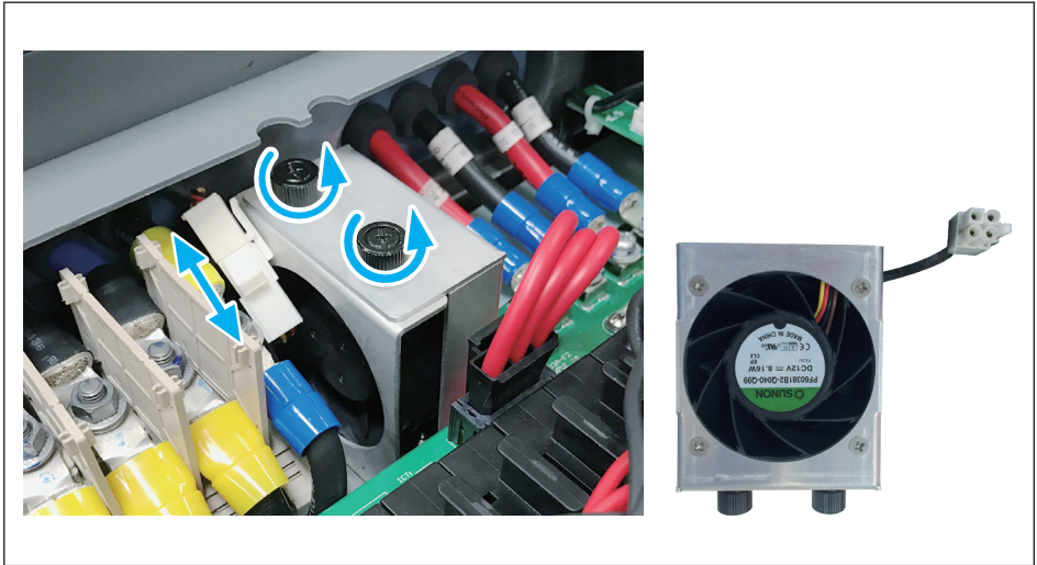
Figure 5-13 : Disassembling fan inside the wiring box compartment (M88H_122 only)
