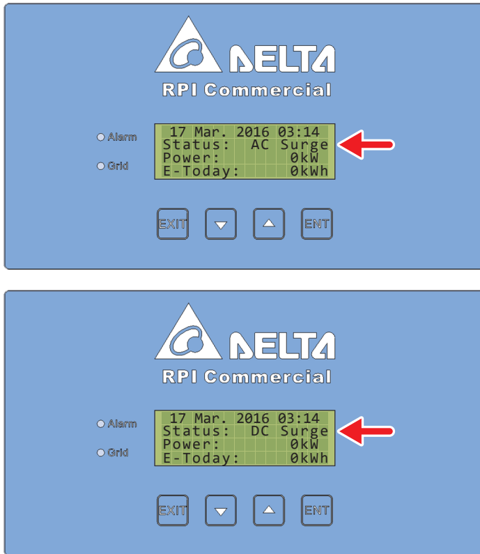
Figure 5-4: Display Indicating AC and DC SPD failure
