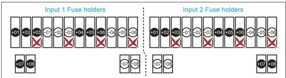
Figure 3-26: Prohibited fuse location using 20A fuse
