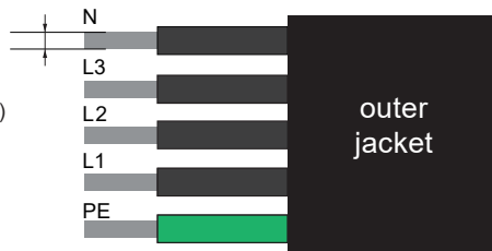
Figure 3-13: Size of AC conductors
