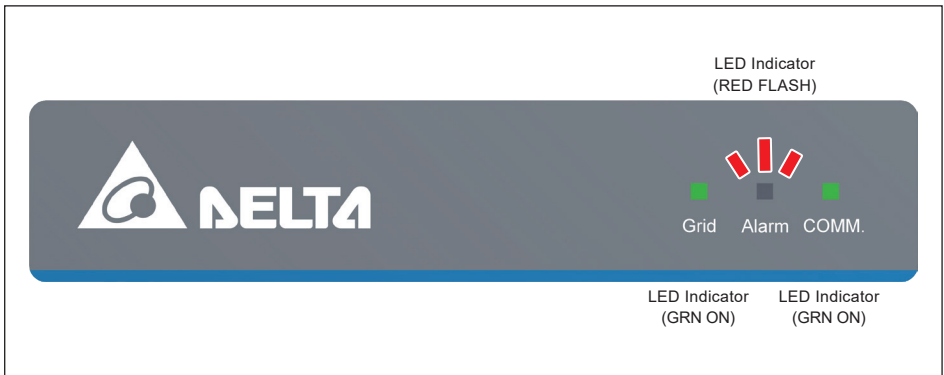
Figure 5-5: Display Indicating AC and DC SPD failure
