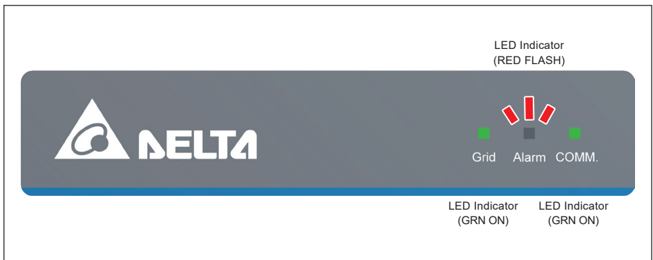
Figure 5-5: Display Indicating AC and DC SPD failure
