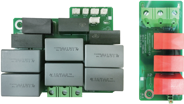
Figure 5-4: AC and DC SPD modules
