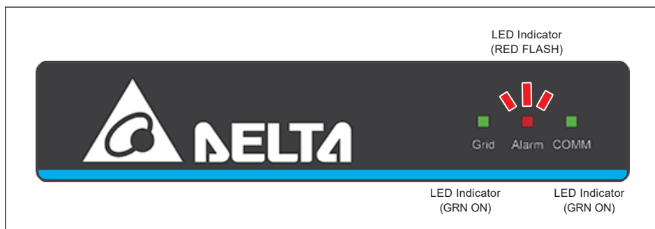
Figure 5-5: Display Indicating AC and DC SPD failure
