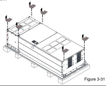
Loosen the six M6 screws and the iron plates (see the figure below). You can use the removed screws and iron plates to fix the drive from outside.
