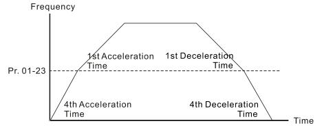
1st/4th Acceleration/Deceleration Frequency Switching
