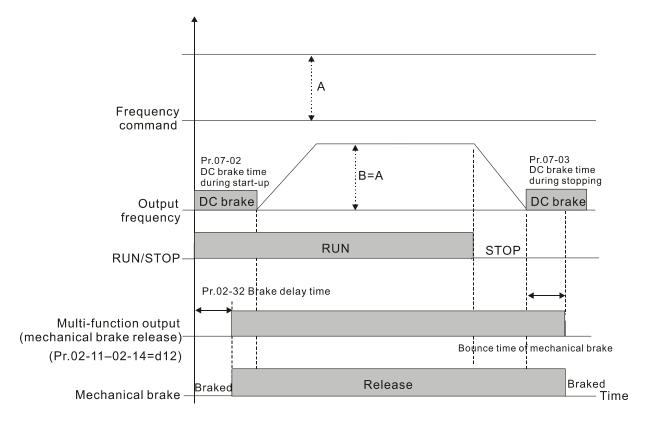
This parameter is invalid if it is used without DC brake. Refer to the following operation timing.
