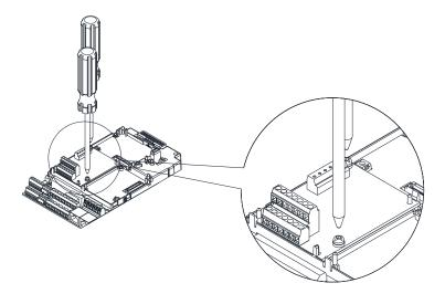
Remove the two screws as shown in the figure on the left.
