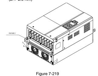
6. Tighten 5 screws (as shown in the figure below). Screw torque: 24-26 kg-cm / (20.8-22.6 lb-in.) / (2.4-2.5 Nm)
