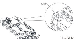
Twist to open the other clip to remove the PCB, as shown in the figure on the left.
