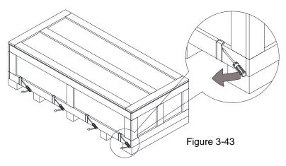
Remove the top cover, take out the EPEs, rubber and the manual.
