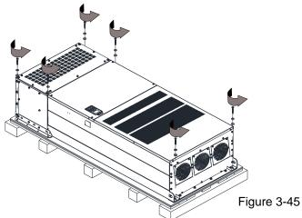
Loosen the six M6 screws and the iron plates (see the figure below). You can use the removed screws and iron plates to fix the drive from the outside.
