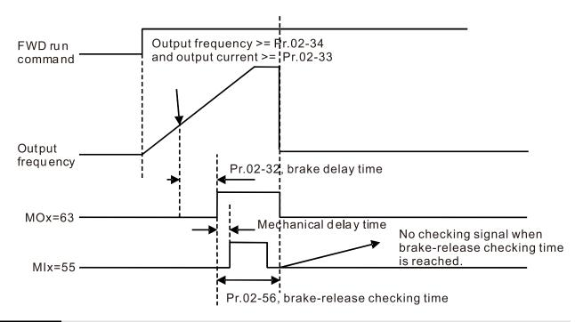
Multi-Function Output Terminal (Function 42): Brake Current Check Point Default: 0
