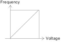
Fcmd=[(ay±bias)\*gain]\*  $\frac{\text{Fmax}(01-00)}{10\text{V or }16\text{mA or }20\text{mA}}$
