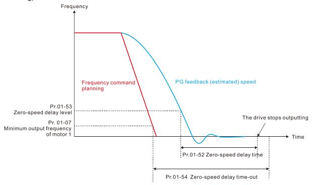
The motor actual speed does not reach the Pr.01-53 level in Pr.01-54 setting time:
