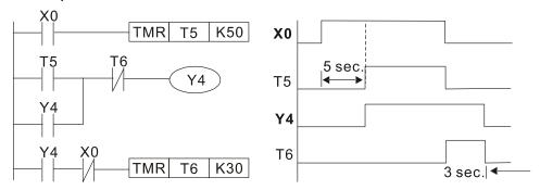
Example 12: Extended timing circuit
