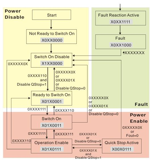
Set command 6040=0xE, and then set another command 6040=0xF. Then you can switch the motor drive to Operation Enable. The Index 605A determines the lines from Operation Enable when the control mode changes from Quick Stop Active. When the setting value is 1–3, both direction lines are active, but when the setting value of 605A is not 1–3, once the motor drive is switched to Quick Stop Active, it is not able to switch back to Operation Enable.)
