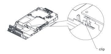
As shown in the figure on the left. Twist to open the other clip to remove the PCB.
