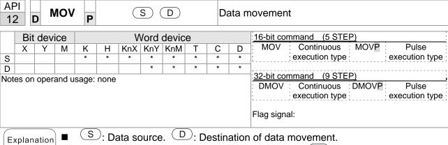
■ When this command is executed, the content of S will be directly moved to D. When the command is not executed, the content of D will not change.
