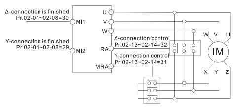
Y-Δ connection switch: can be used for wide range motor
