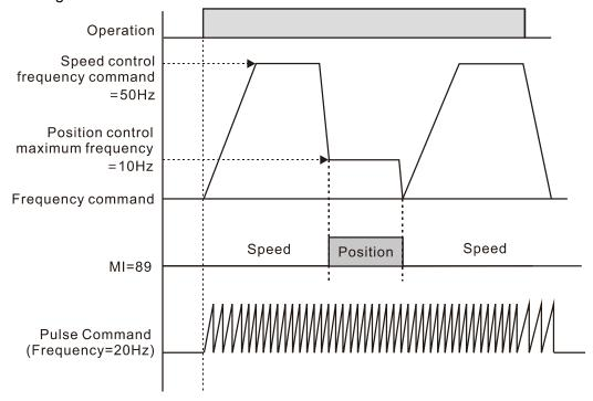
When setting bit8 = 0 (point-to-point position control) to Pr.11-00, the speed of movement among every position is based on this parameter.
