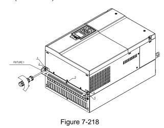
5. Tighten 4 screws (as shown in the figure below). Screw torque: 24-26 kg-cm / (20.8-22.6 lb-in.) / (2.4-2.5 Nm)
