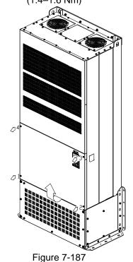
2. Loosen the screw 1–8 and remove the top cover. Screw torque: 24-26kg-cm / (20.8-22.6 lb-in.) / (2.4-2.5 Nm)
