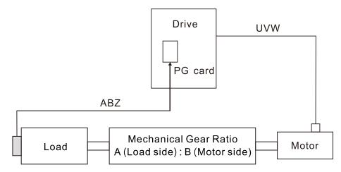
3. <u>Fully-closed loop control method: Type A</u> (Encoder is installed at the motor side, and Z-phase signal comes from the load side)
