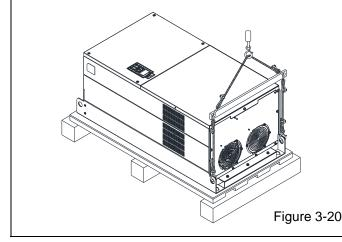
Lift the drive by hooking the lifting hole. It is now ready for installation.
