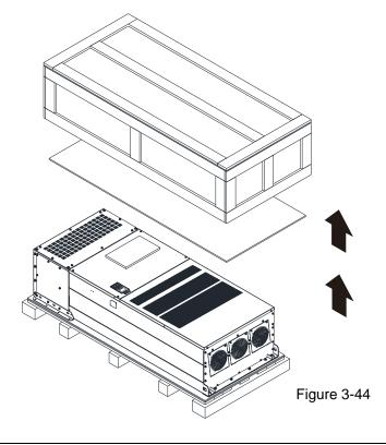
Loosen the six screws fasten the drive on the pallet, and then remove six metal washers and six plastic washers. See the figure below.
