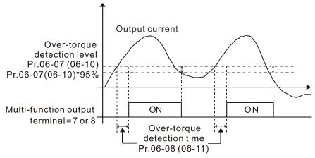
When you set Pr.06-06 or Pr.06-09 to 2 or 4, an ot1 / ot2 warning displays and the drive stops running after over-torque detection. The drive does not run until you manually reset it.
