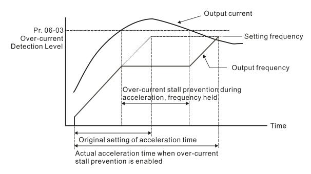
Refer to Pr.06-16 for more details of stall level in flux weakening region. The protection curve is as follows:
