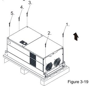
Loosen the 12 screws fasten the drive on the pallet, and then remove the wood plates and conduit box.
