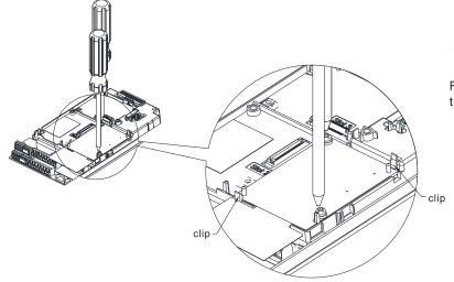
Remove the two screws as shown in the figure on the left.
