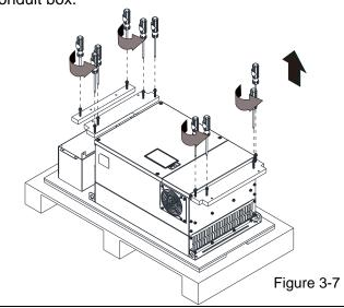
Lift the drive by hooking the lifting hole. It is now ready for installation.
