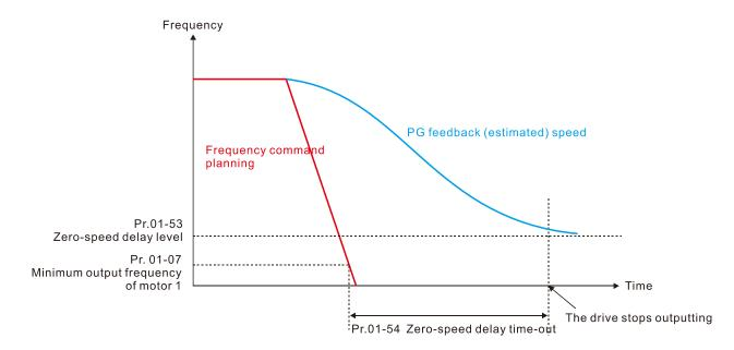
The motor actual speed reaches the Pr.01-53 level in Pr.01-54 setting time, but does not reach to 0 Hz in Pr.01-54 setting time:
