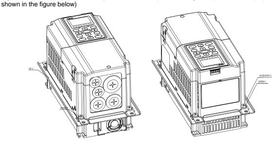
Figure 7-202 Plate installation, place 4 of the screw \*4 (M6) through accessory 2 & 3 and the plate then tighten the screws.
