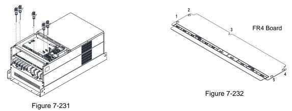
3. Loosen the upper M8 nuts (1–6) with a sleeve wrench (12mm of the sleeve). M8 Torque: 90kg / (78.1 lb-in) / (8.8 Nm)
