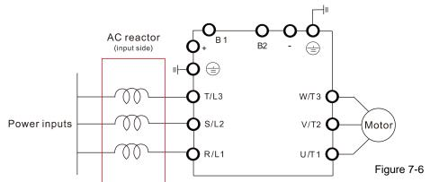
Wiring of AC input reactor
