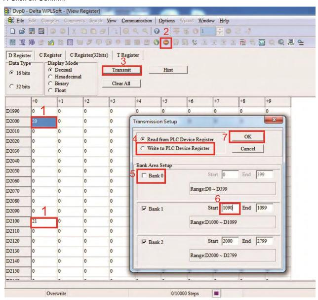
Another method can be used to set D1091: Determine which of slave stations 0 to 7 will not be needed, and set the corresponding bits to 0. For instance, if it is not necessary to control slave stations 2, 6 and 7, merely set D1091 = 003B, and the setting method is the same as described above: Use WPL to initiate communications > use register edit (T C D) function to perform settings.
