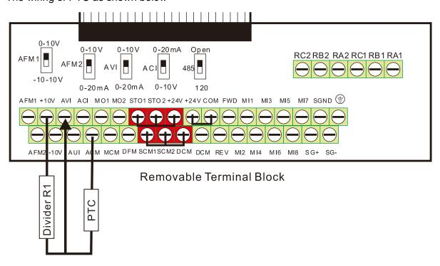
The wiring of KTY-84 as shown below
