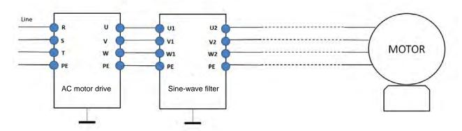
Figure 7-37 Wiring of non-shielded cable
