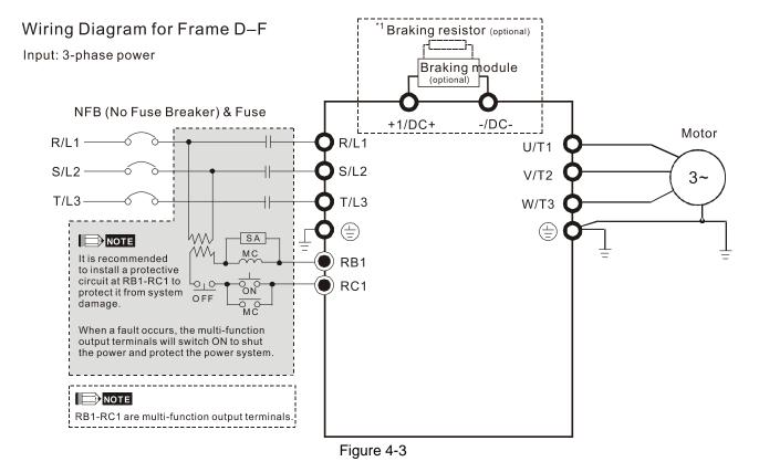
NOTE: \*1 means that refer to Section 7-1 for brake units and resistors selection.
