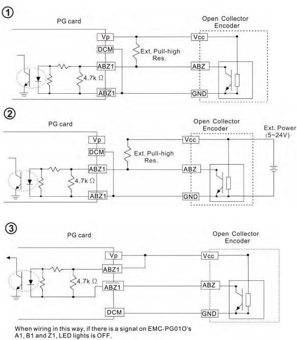
If A1, B1 and Z1 have no signals, LED lights is ON.
