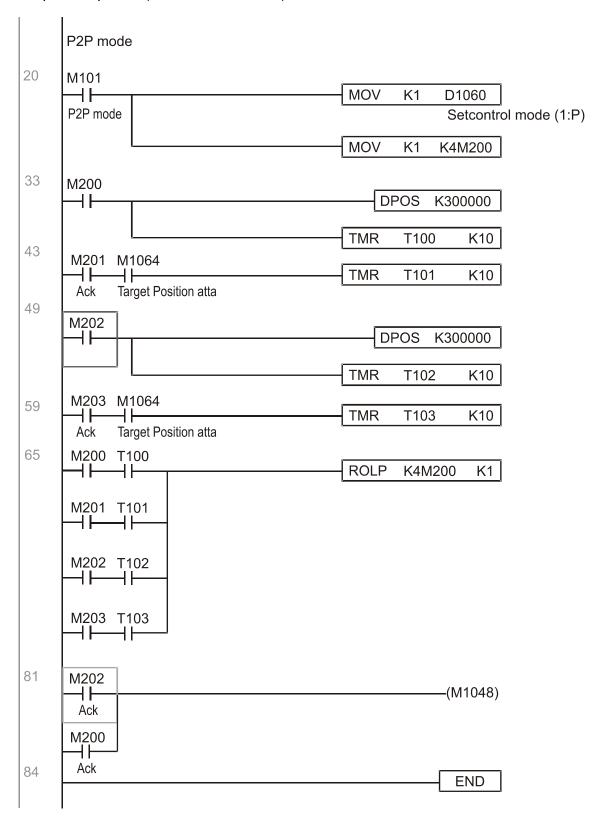
**NOTE:** If homing is not needed in an application, the first and second parts can be skipped. However, the M1040 condition from Part 1 must be included, and the writing method in Part 1 involve the use of X2 to achieve direct access. In addition, when M101 is used at the beginning of Part 3 to set the control mode, it can be rewritten as M1002, which will put the PLC immediately into the position mode when it starts running.
