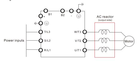
Figure 7-25 Wiring of AC output reactor
