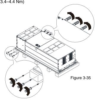
Tighten the six M6 screws that removed in the figure 3-32 back, see the figure below.
