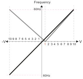
Pr.00-21=0 (Digital keypad control and run in FWD direction) Pr.03-05 Analog Positive Voltage Input Bias (AUI) = 10%
