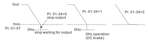
In FOCPG mode, when Pr.01-34 is set to 2, the AC motor drive operates according to this setting.
