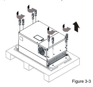
Loosen the ten screws fasten the drive on the pallet, and then remove the wood plates and the conduit box.
