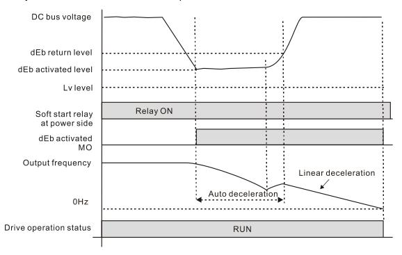
Situation 2: Momentary power loss, or too low and unstable power voltage, or power supply sliding down because of sudden heavy load.
