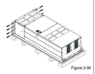
Tighten the six M6 screws back, see the figure below. Torque: 35–45 kg-cm / (30.38–39.06 lb-in) / (3.4–4.4 Nm)
