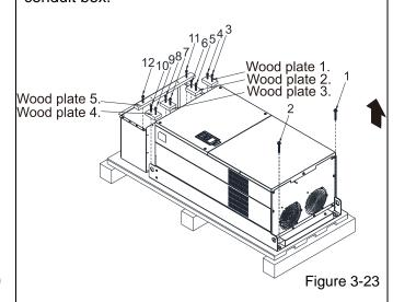
Lift the drive by hooking the lifting hole. It is now ready for installation.
