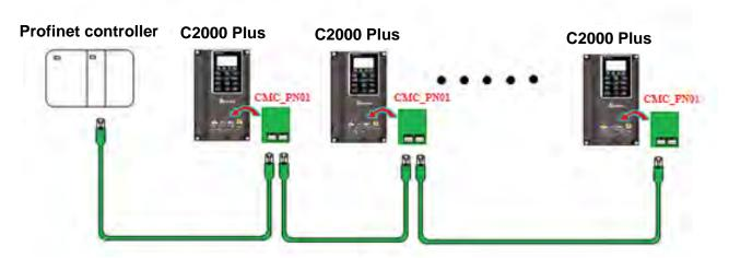
When the installation is finished, supply electricity to the drive. The Pr.09-60 of the drive should be able to display "PROFINET" with a current value of 12. If not, make sure your version of the drive is correct (C2000 Plus needs V3.05 or later versions) and the communication card is correctly connected.
