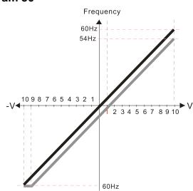
Pr.00-21=0 (Digital keypad control and run in FWD direction) Pr.03-05 Analog Positive Voltage Input Bias (AUI) = 10% Pr.03-07~03-09 (Positive/Negative Bias Mode)
