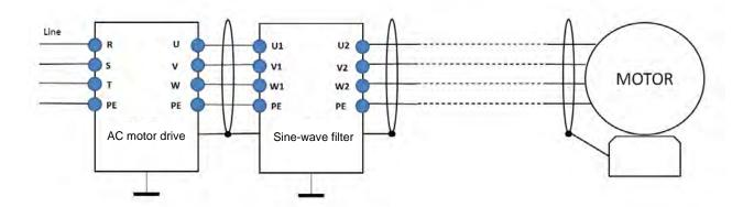
Figure 7-38 Wiring of shielded cable
