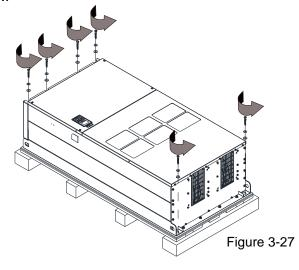
Lift the drive by hooking the lifting hole. It is now ready for installation.  $\hfill\Box$
