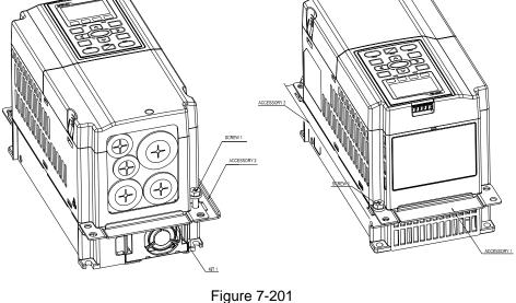
Tighten screw\*2 (M6) and accessory 2 & 3. Screw torque: 25–30 kg-cm / (21.7–26 lb-in.) / (2.5–2.9 Nm)
