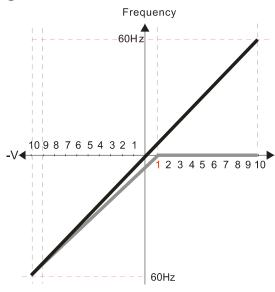
Pr.00-21=0 (Digital keypad control and run in FWD direction)
