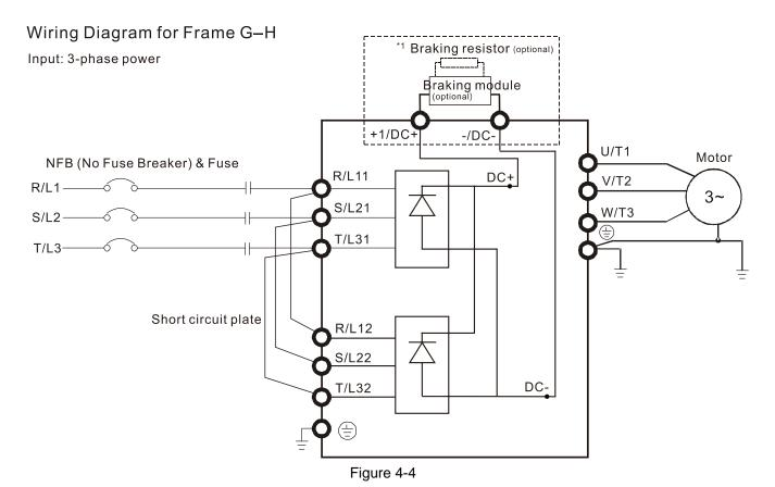
Wiring Diagram for Frame G-H
