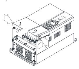
2. Loosen screw 3, press the tab on the right and the left to remove the cover. Screw 3 Torque: 6–8 kg-cm / (5.2–6.9 lb-in.) / (0.6–0.8 Nm)
