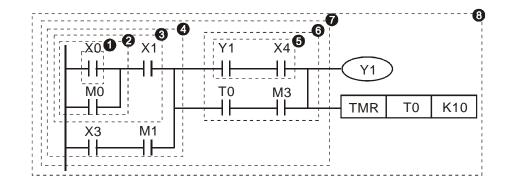
Explanation of basic structure of ladder diagrams
