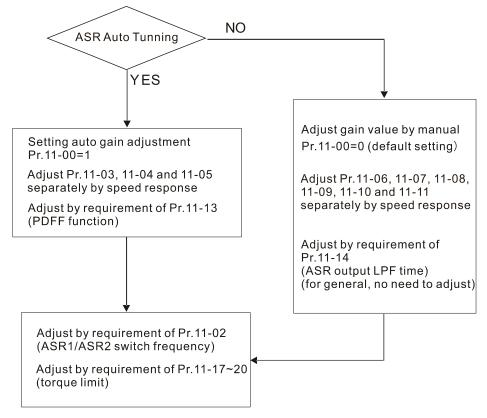
When the drive needs to keep a certain torque at zero-speed, or it needs a steady frequency output at extremely low speed, increase Pr.11-05 zero-speed bandwidth appropriately. When the speed is in high-speed area, if the output current trembles seriously and makes the drive vibrate, then decrease the high-speed bandwidth.
