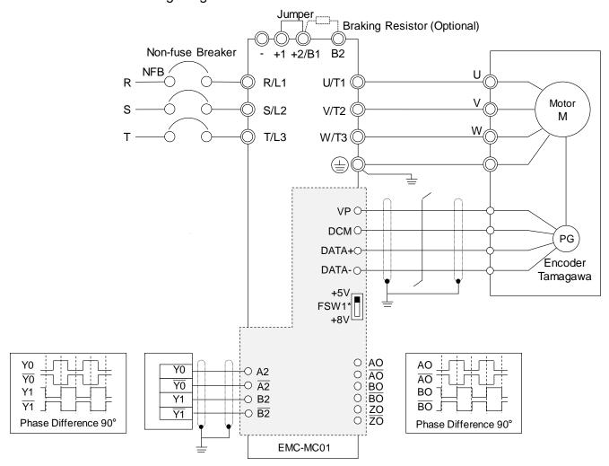
**NOTE:** The current input voltage for Tamagawa encoder is +5V, ensure to switch to +5V before the installation. The voltage +8V is reserved for the power demand of other encoders in the future.
