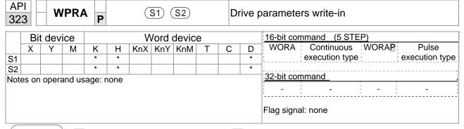
S1: Data that is going to write in S2: Parameter address of the write-in data
