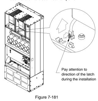
2. Loosen the screw 5–12 and remove the top cover. Screw torque: 24–26 kg-cm / (20.8–22.6 lb-in.) / (2.4–2.5 Nm)
