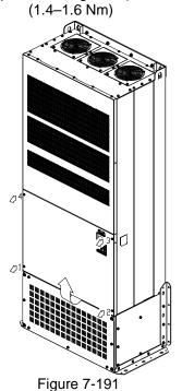
2. Loosen the screw 1–8 and remove the top cover. Screw torque: 24–26kg-cm / (20.8–22.6 lb-in.) / (2.4–2.5 Nm)
