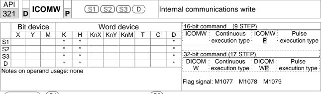
S1: Selection of slave device. S2: Device selection (0: converter, 1: internal PLC). S3: Read address. D: Saving target.
