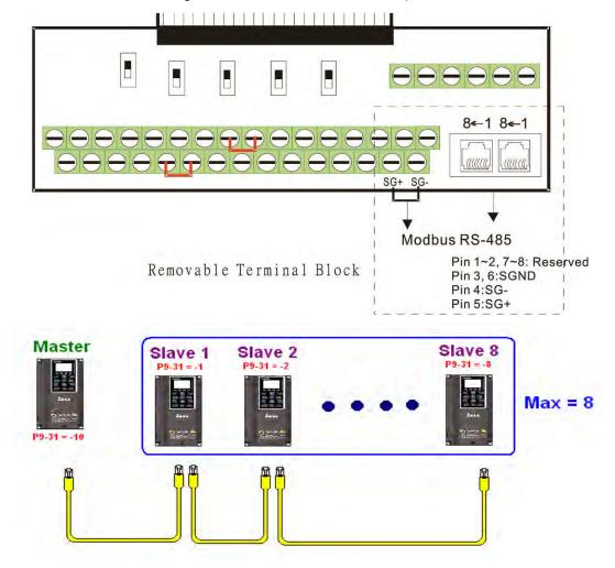
Master programming: In a program, D1110 can be used to define a slave station to be controlled (1–8, if set as 0, can jump between 8 stations). Afterwards, M1035 is set as 1, and the memory positions of the master and slave stations will correspond. At this time, it is only necessary to send commands to the correlation slave station address to control that station. The following is a register table connected with internal communications:
