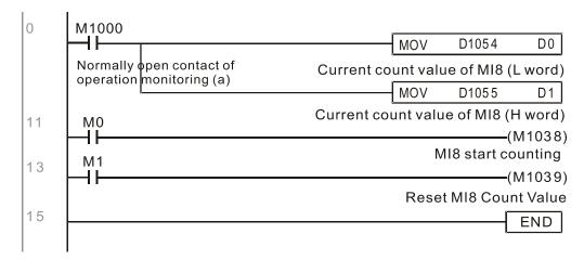
**NOTE:** When the PLC program defines MI8 for use as a high-speed counter, and also for use in PLC procedures, it must be written to M1038 or M1039, and the original MI8 functions will be disabled.
