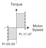
Forward Speed Limit (Torque Mode)
