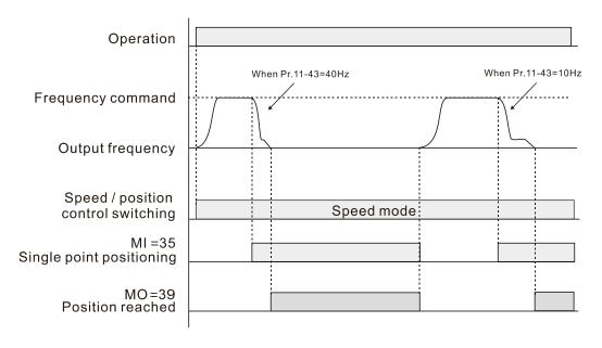
If the multi-function input terminal MIx = 89 (position / speed mode switch) is enabled under the speed mode, the drive executes pulse-train positioning according to Pr.11-43 setting, as shown in the diagram below.
