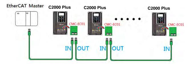
When the hardware is installed and power on, check for the display. The current set value of Pr.09-60 will be 6, and shows "EtherCAT" on the display. If the above information does not show on the display, check the version of C2000 Plus (V3.05 and later) and the connection of the card.
