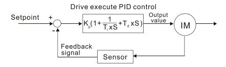
K<sub>P</sub> Proportional Gain (P), T<sub>i</sub> Integral Time (I), T<sub>d</sub> Differential Time (D), S Calculation
