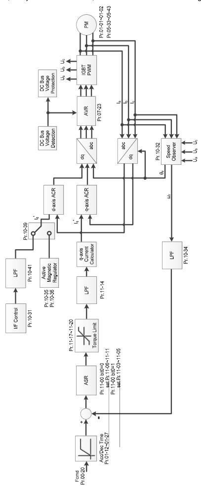
$\square$  When Pr.00-10 = 0, and you set Pr.00-11 to 7, IPM FOC sensorless control diagram is as follows:
