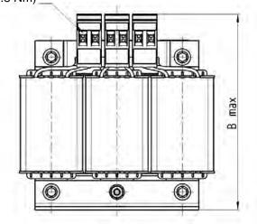
Screw length must not interfere with the mounting holes
