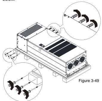
Tighten the six M6 screws back, see the figure below.
