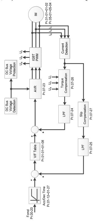
$\square$  When Pr.00-10 = 0, and you set Pr.00-11 to 1, the V/F control + encoder diagram is as follows.
