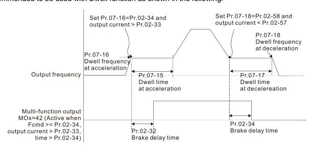
When using the crane application and MOx = 42, Pr.02-34 must be larger than Pr.02-58; Pr.02-33 must be larger than Pr.02-57.
