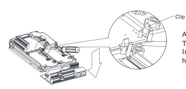
As shown in the figure on the left. Twist to open the clip. Insert a slot type screwdriver into the hollow to prize the PCB off the clip.
