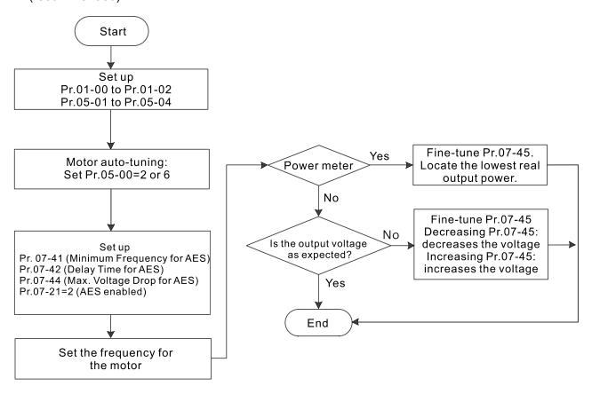
See below for the flowchart of AES adjustment without motor parameter auto-tuning (not recommended):
