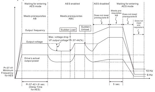
The energy-saving function is invalid during the drive's acceleration and deceleration. To make it valid, the prerequisites need to be verified again.
