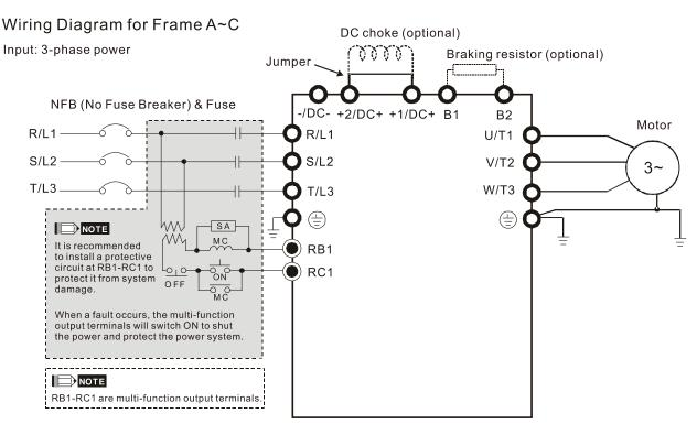
Figure 7-23 Wiring of DC reactor
