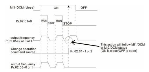
When you set Pr.02.05 = 1 or 3, it does not guarantee that the drive will never run. Be careful when using this function because the switch may bounce due to mechanical vibration or defective switch parts.
