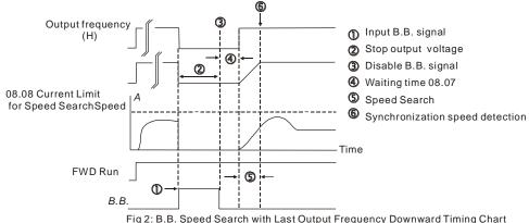
Fig 2: B.B. Speed Search with Last Output Frequency Downward Timing Chart (Speed Search Current doesn't Attain Speed Search Level)
