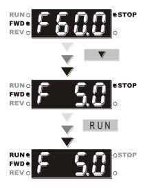
If the results of trial run are normal, increase the operating frequency to continue the trial run. If the trial run still goes normally, then you can start the formal run.
