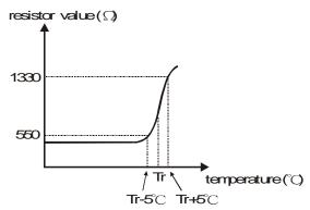
Refer to the following calculation when Pr.07.14 is set to 2.4 and motor temperature overheating protection level is 1330  $\Omega$ :
