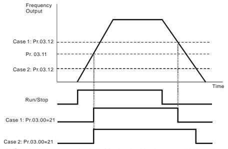
Pr.03.00 multi-function output terminal 21: Mechanical brake control: When the output frequency reaches Pr.03.11 (Mechanical brake release frequency), this terminal is closed (ON); when the output frequency reaches Pr.03.12 (Mechanical brake active frequency), this terminal is OFF.
