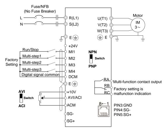
NOTE Terminal SG+,SG- are joined to PIN5,PIN4 of RJ45 Connector
