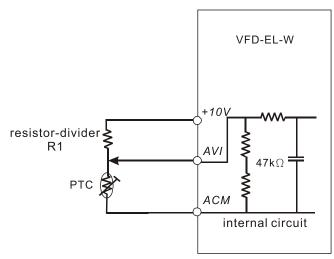
Take the standard PTC thermistor as an example: if the protection level is 1330  $\Omega$ , the actual voltage between +10V-ACM is 10.5 V and divider resistance R1 is 4.4k  $\Omega$ .
