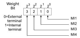
When setting this parameter, covert bit3-bit0 that represent the status of MI4-MI1 from binary to decimal, and then set this parameter. Set MI3 and MI4 as internal terminals; set MI1 and MI2 as external terminals. Pr.04.27 should be set to 12.
