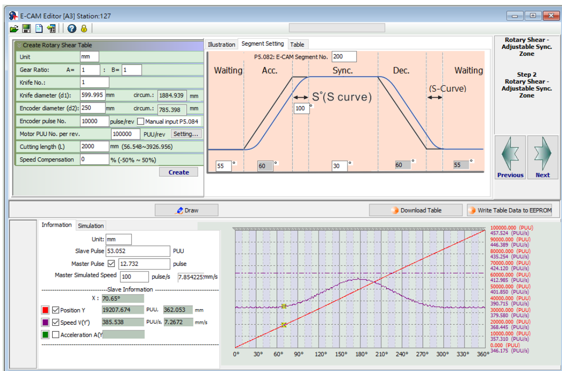
Figure 7.3.7.11 ASDA-Soft setting interface for [Rotary Shear - Adjustable Sync. Zone]
