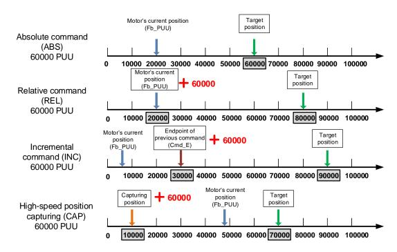
Figure 7.1.3.3.3 Four types of Position command
