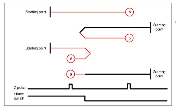
Method 7: homing on the positive limit switch, rising edge of home switch, and Z pulse
