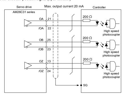
Note: the pin definition of the communication type models is different from that of the L model. Communication type model pins: OA (1), /OA (2), OB (11), /OB (12), OZ (3), and /OZ (4).
