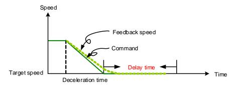
Figure 7.1.3.2.2 Parameters for PR mode speed control
