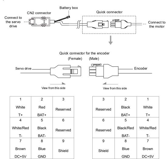
Note: the wire colors of the ASDA-B3 servo drive are for reference only. Refer to the actual servo drive.
