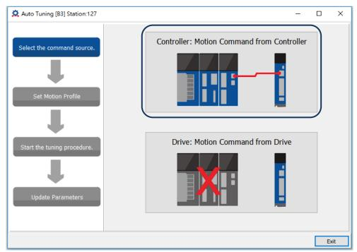
Suggestions: set the motor to operate at least one cycle in both positive and negative directions. The delay time for reaching the positions in both positive and negative directions should not be less than 1,000 ms with the running speed no less than 500 rpm.
