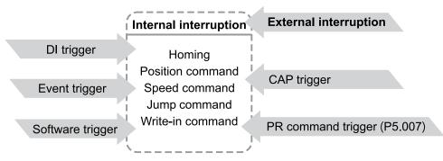
Figure 7.1.6.5 Internal and external interruption
