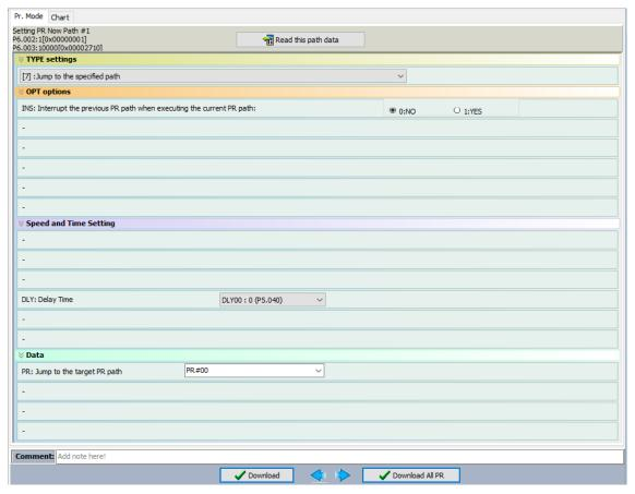
Figure 7.1.3.4.2 PR Mode Jump command screen in ASDA-Soft
