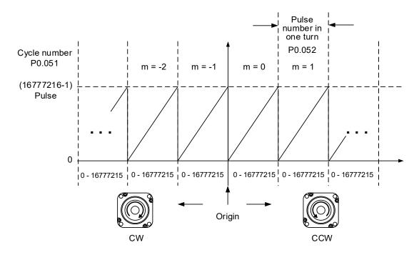
Figure 10.3.2.1 Absolute position for pulse number
