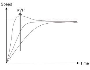
The higher the KVP value, the larger the bandwidth. The time of the speed increase will also be shorter. However, if the value is set too high, the phase margin is too small. The effect is not as good as KVI for the steady-state error but is better for the effect on following error.
