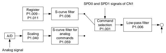
The upper path is the command from the register and the lower one is the command from the external analog voltage that you can select with the status of SPD0 and SPD1, and P1.001 (S or Sz). In this condition, the S-curve and low-pass filters are applied to achieve a smoother response.
