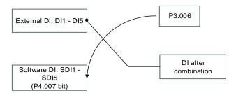
Read parameters: shows the DI status after combining external DI and software DI.
