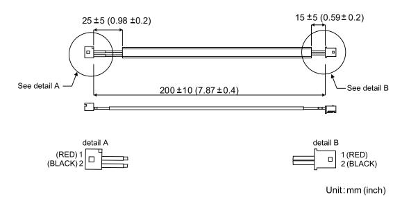
Battery box cable for self-wiring (part number: 3864850600)
