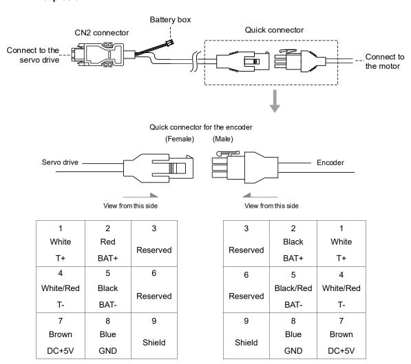
Note: the wire colors of the ASDA-B3 servo drive are for reference only. Refer to the actual servo drive.
