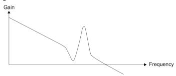
When the value of P2.025 is increased from 0, BW becomes smaller, as shown in the following figure. Although it solves the problem of the resonance frequency, the response bandwidth and phase margin are reduced.
