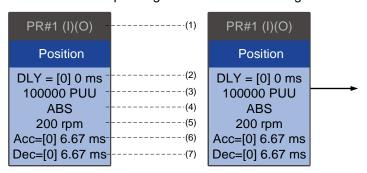
Figure 7.1.4.4 Position command display
