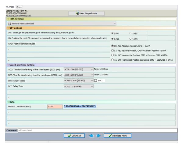
Figure 7.1.3.3.1 PR mode Position control screen in ASDA-Soft
