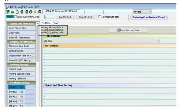
Figure 7.1.2 PR Mode interface in ASDA-Soft
