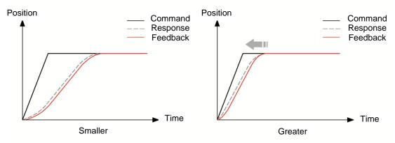
Figure 5.3.6.1 Adjust the command response gain
