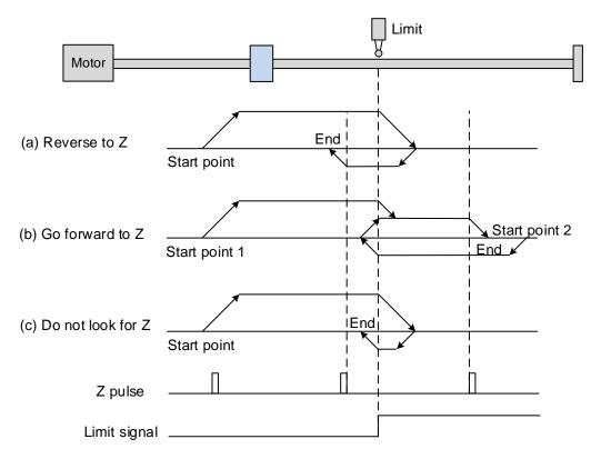
(a) If you set the servo to look for the Z pulse in the reverse direction, the servo operates at high speed (first speed setting) and then decelerates once it reaches the limit (rising-edge triggered). Then the servo switches to low speed (second speed setting) to look for the Z pulse in the reverse direction. When the servo finds the Z pulse, it decelerates to a stop, completing the homing procedure.
