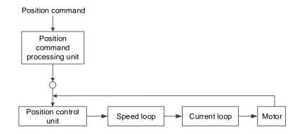
For better control, the pulse signals are processed by the Position command processing unit. The structure is shown in the following diagram.
