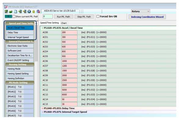
Figure 7.1.1.2 ASDA-Soft interface for shared PR parameter data
