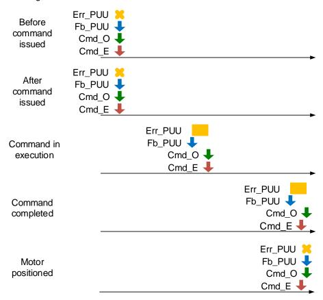
Figure 7.1.3.1.3 Homing mode and monitoring variables
