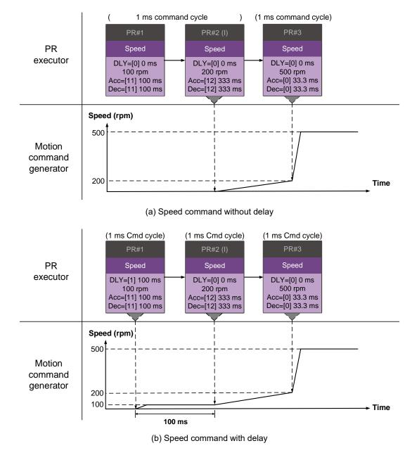
Figure 7.1.6.8 Internal interruption - Speed command
