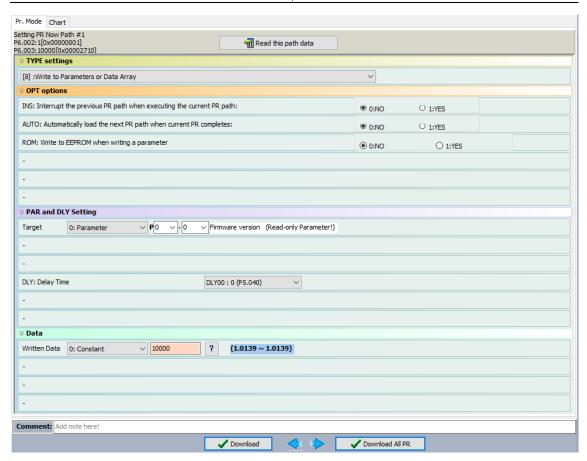
Figure 7.1.3.5.1 PR mode Write command screen in ASDA-Soft
