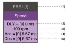
Figure 7.1.4.3 Speed command display
