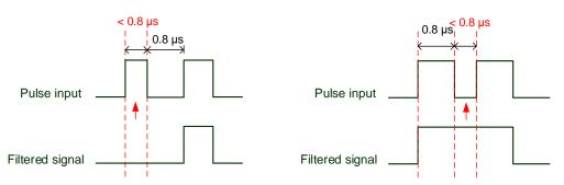
If the first pulse width is smaller than 0.8  $\mu$ s, it may be filtered out, and thus two input pulses will be regarded as one pulse. If the pulse width is smaller than 0.2  $\mu$ s, it will be filtered out.
