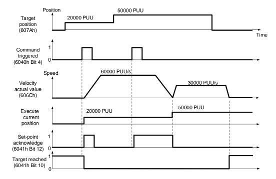
■ When 6040h Bit 5 is set to 1, the command to take immediate effect is enabled (only valid in Profile Position Mode).
