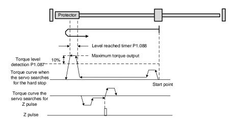
Note: the actual maximum torque output of the motor is 10% greater than the detected torque level (P1.087).
