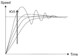
The higher the KVI value, the larger the low-frequency gain. It shortens the time for the steady-state error to reduce to zero. However, it does not significantly reduce the following error.
