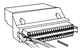
(2) Insert the stripped wire into the pin and withdraw the screwdriver to complete the wiring.
