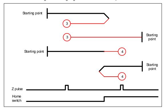
Methods 5 and 6: homing on the falling edge of home switch and Z pulse
