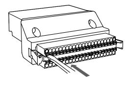
(1) The CN1 quick connector has multiple spring terminals. Determine which terminal is to be wired in advance. Use a flathead screwdriver to press the spring down to open the pin.
