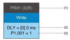
Figure 7.1.4.6 Write command display
