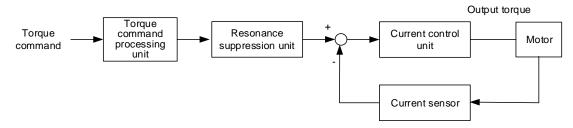
The Torque command processing unit selects the command source (see Section 6.4.1), including the scaling parameter (P1.041) for rotation speed and S-curve parameter for smoothing the torque. The current control unit manages the gain parameters for the servo drive and calculates the current for servo motor in real-time; you can only set this by commands.
