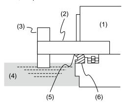
(1) Servo motor; (2) Motor shaft; (3) Gear; (4) Oil; (5) Oil seal lip; (6) Oil seal
