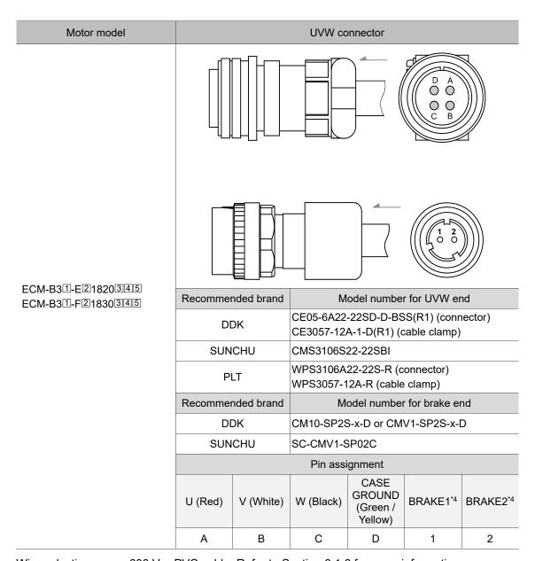
Wire selection: use a 600  $V_{\text{AC}}$  PVC cable. Refer to Section 3.1.6 for more information.
