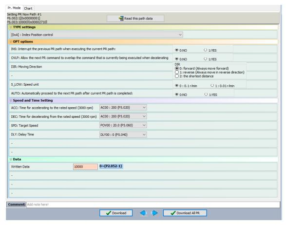
Figure 7.1.3.6.3 PR mode Index Position screen in ASDA-Soft
