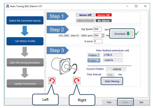
Step 3: Wait until the tuning progress bar reaches 100%, after which a window with "Auto tuning completed." appears. Click **OK** to continue.
