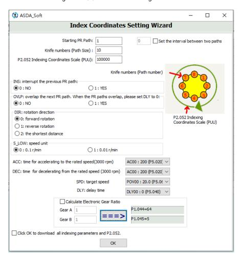
Figure 7.1.3.6.2 Index Coordinates Setting Wizard in PR mode
