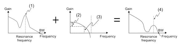
(1) Resonance point; (2) Attenuation rate (-3 dB); (3) Low-pass filter (Cutoff frequency of low-pass filter = 1000 / P2.025 Hz); (4) Resonance point suppressed by the low-pass filter
