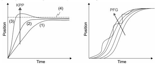
The actual position curve changes from (1) to (3) with the increase in the KPP value. (4) stands for the Position command.
