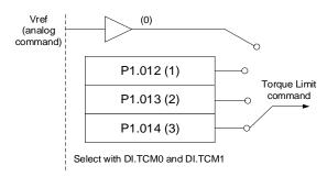
When using the Torque Limit function, set this parameter to 1 to limit the torque permanently without occupying a DI setting. Alternatively, you can enable or disable the limit function with DI.TRQLM, which is more flexible, but the setting then occupies a DI setting. You can enable the Torque Limit function with either P1.002 or DI.
