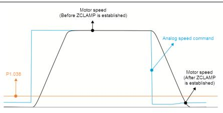
Bit 10 = 1 and command source is the internal register. ZCLAMP function uses the register Speed command with acceleration or deceleration to determine if this function should be enabled. When ZCLAMP conditions are met, the motor speed is set to 0 rpm.
