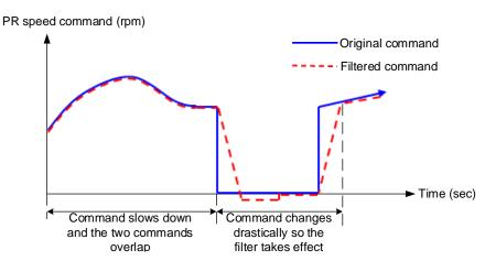
Note: if the command does not slow down, the following error of the internal position exceeds the allowable range and then triggers AL404.
