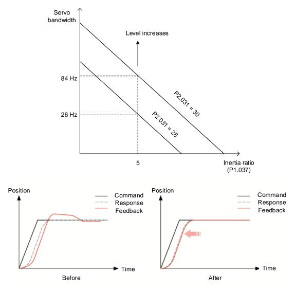
Figure 5.3.5.1 Adjust the bandwidth response level
