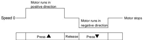
If the motor does not run, check if the wiring between U, V, W and encoder cable is correct.
