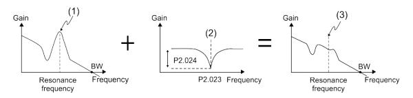
(1) Resonance point; (2) Notch filter; (3) Resonance point suppressed by the Notch filter
