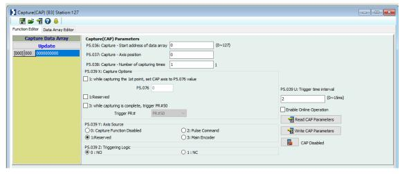
Figure 7.2.2.2 Capture function screen in ASDA-Soft
