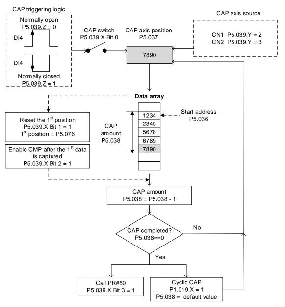
Figure 7.2.2.1 Flowchart for high-speed position capturing
