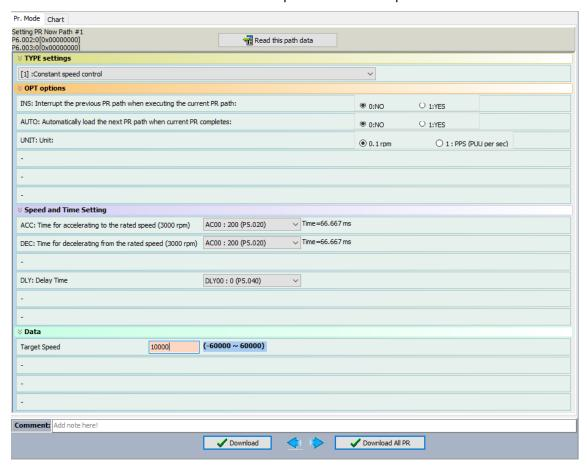
Figure 7.1.3.2.1 PR mode Speed control screen in ASDA-Soft
