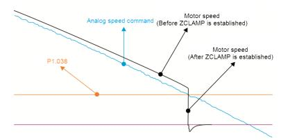
Bit 10 = 0 and command source is the internal register. The ZCLAMP function uses the register Speed command with acceleration or deceleration to determine if this function should be enabled. The motor is clamped at the position where ZCLAMP conditions are met.
