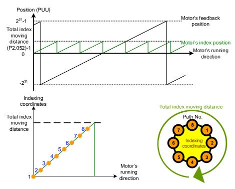
Figure 7.1.3.6.1 PR mode indexing coordinates
