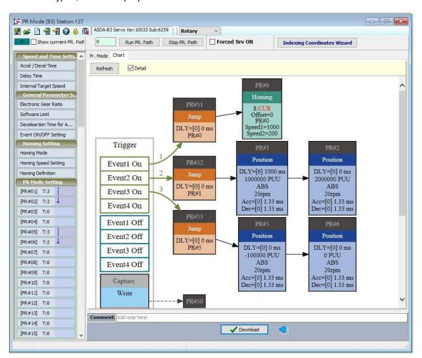
Figure 7.1.3 PR Diagram display in ASDA-Soft
