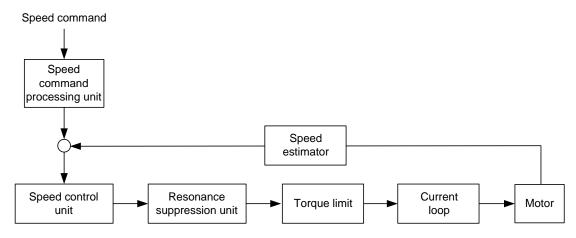
The Speed command processing unit selects the command source (see Section 6.3.1), including the scaling parameter (P1.040) for maximum rotation speed corresponding to the analog voltage and the S-curve parameter for smoothing the speed. The Speed control unit manages the gain parameters for the servo drive and calculates the current command for servo motor in real-time. The Resonance suppression unit suppresses the resonance of the machine.
