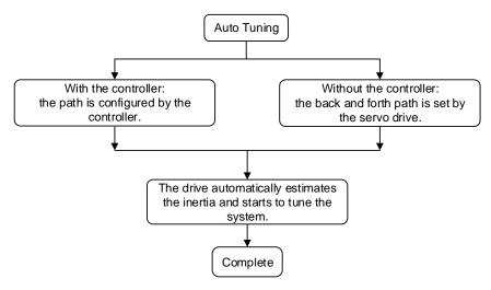
Note: when the path is configured by the controller, make sure the dwell time is added to the operation cycle. Otherwise, AL08B occurs and the servo drive cannot complete auto tuning.
