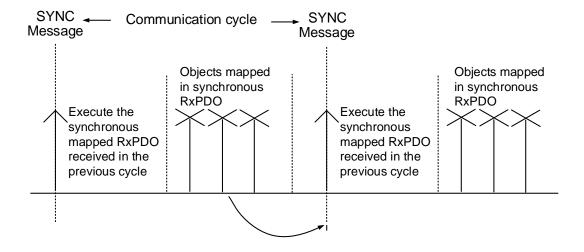
The following figure shows the timing sequence between the servo drive TxPDO transmission and the controller SYNC transmission. The servo drive transmits the TxPDO data to the controller as soon as it receives the SYNC.
