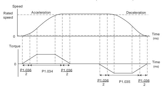
Figure 6.3.3.1 S-curve and time setting
