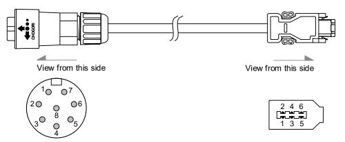
Pin assignment of CN2 connector:
