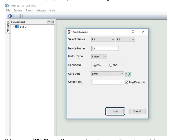
Make sure your ASDA-B3 servo drive, servo motor, and power are all properly connected. Then click **Add** for the ASDA-Soft to be in online mode.
