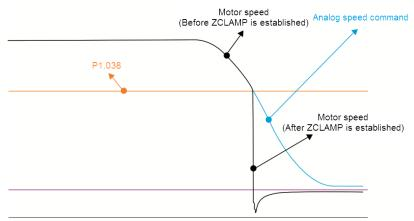
Bit 10 = 1 and command source is the analog voltage.
