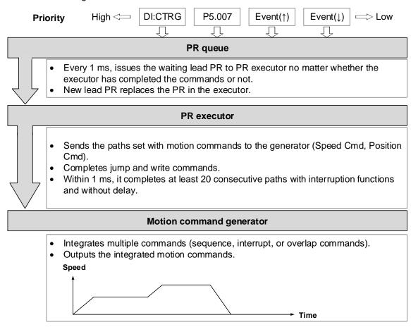
Figure 7.1.6.1 PR execution flow in the ASDA-B3
