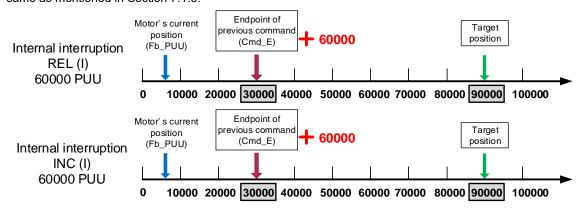
Figure 7.1.6.7 Example of relative and incremental position commands for internal interruption
