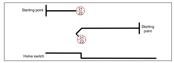
Methods 23 and 24: homing on the positive limit switch and rising edge of home switch
