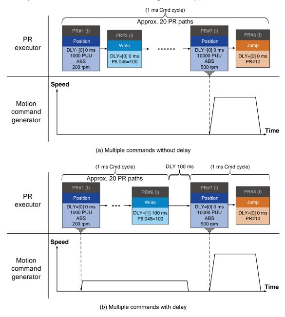
Figure 7.1.6.9 Internal interruption - Multiple commands
