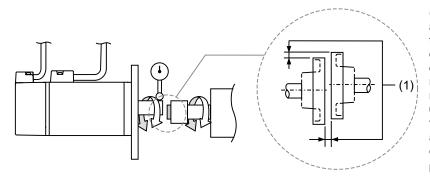
(1) The distance is measured at four different positions on the circumference for the centering precision. The difference between the maximum and minimum measurements should be 0.03 mm or less; even within this range, you can make adjustments to increase the centering precision.
