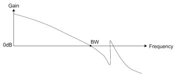
If you know the resonance frequency, you can suppress the resonance by using the Notch filter. The frequency range of the Notch filter is 50 - 5000 Hz and the suppression strength is 0 - 40 dB. If the frequency does not meet the Notch filter conditions, then using the low-pass filter to reduce the resonance is suggested.
