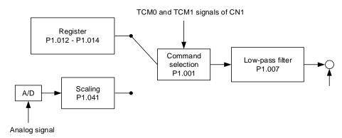
The upper path is the command from the register and the lower one is the command from the external analog voltage that you can select with the status of TCM0 and TCM1, and P1.001 (T or Tz). Adjust the torque with the analog voltage scaling (P1.041) and smooth the response with the low-pass filter (P1.007).
