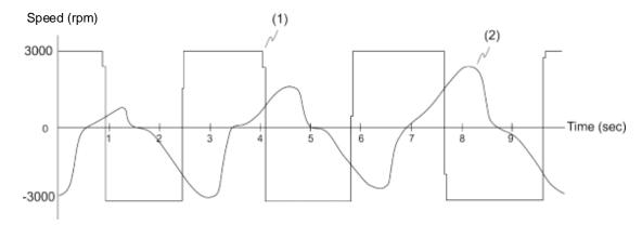
(1) Analog Speed command; (2) Motor speed
