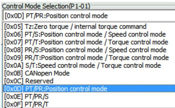
Step 2: Select dual position control mode. The setting block on the left will show as below:
