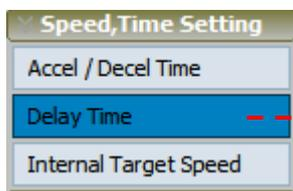
The unit of 16 sets of delay time is ms. Its setting range is from 0 to 32,767 ms.
