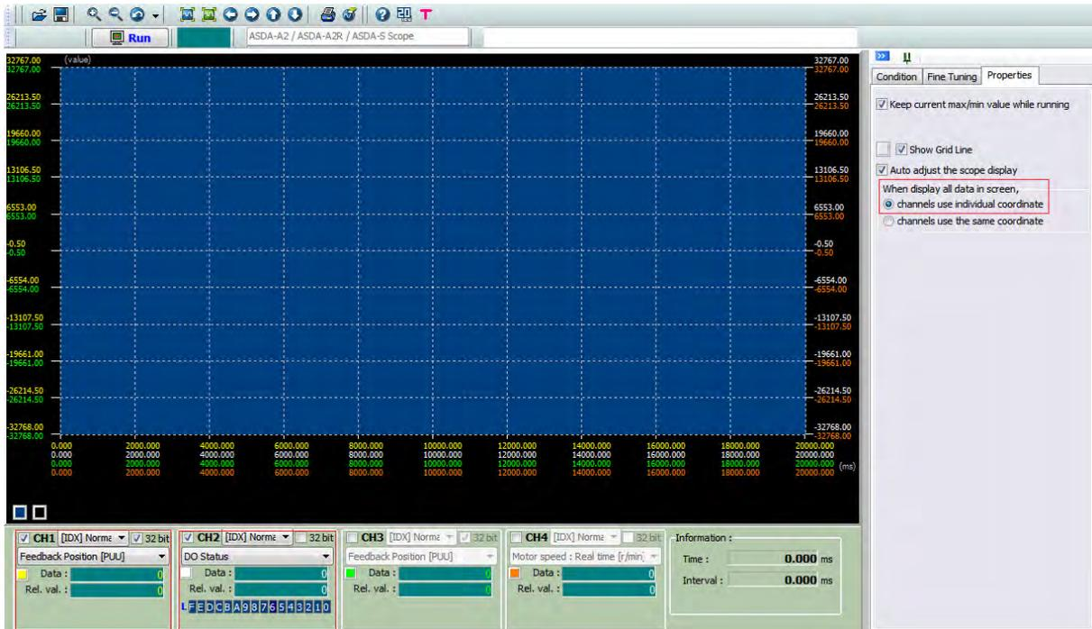
Channel 1: Set as accessing feedback position (PUU). Since the unit of PUU is 32-bit, please check  32 bit.
