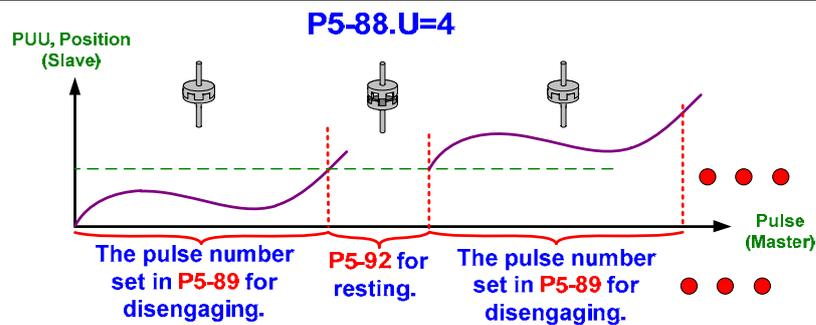
When the setting is complete, click  to download the “Engaged condition” into the servo drive. As the previous description, if it is not connected to the master axis, users can select the time axis (1ms) as master axis to drive slave axis so as to simulate E-Cam operation.
