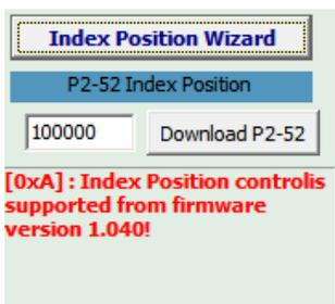
: Users can adjust the setting of indexing range.
