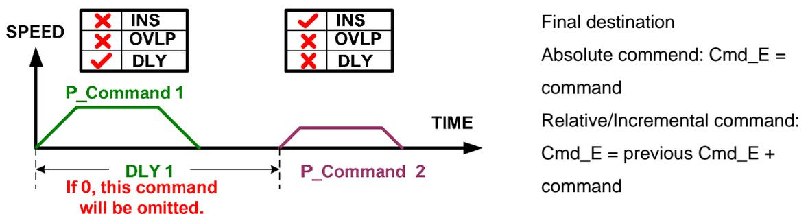
In this diagram, the previous PR is speed control. If the speed command 1 is set with delay time and will auto move to the next PR (speed control is set to AUTO), the position command will be executed when the delay time is reached. Speed command 1 and position command 2 will be executed in sequence smoothly.
