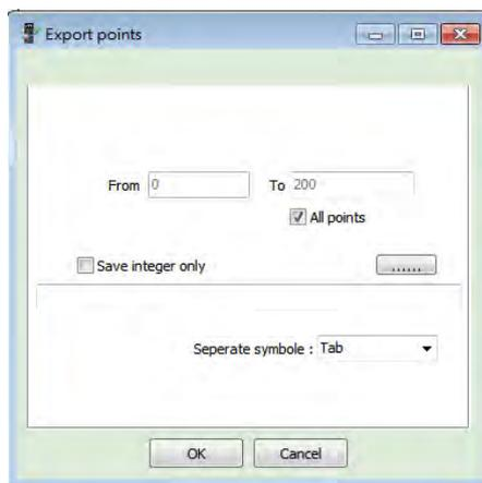
Then, setup the range. Cancel the option of All points in this window. Manually enter the range from 0 to 200.
