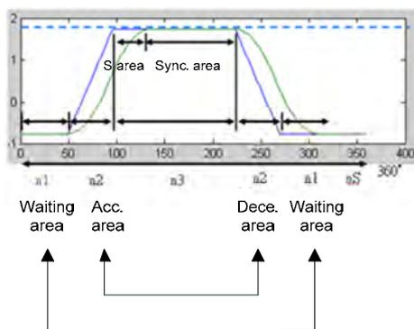
The setting method of waiting area: The initial value in waiting area is 0. It is because the acceleration/deceleration curve is smoother than no one in this status. The bigger value in waiting area, the shorter distance motor can run in reverse direction and the speed change is severer. It is easier to cause current overload.
