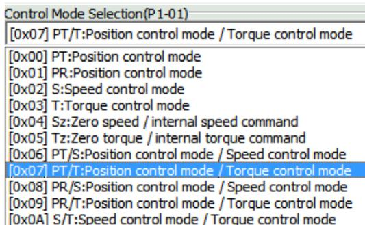
Step 2: Select Position control mode / Torque control mode, the setting block on the left will show as below:
