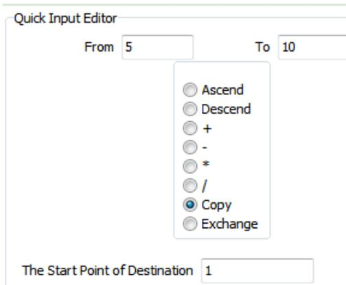
Copy the value from 5 to 10 to the target position starting from 1.
