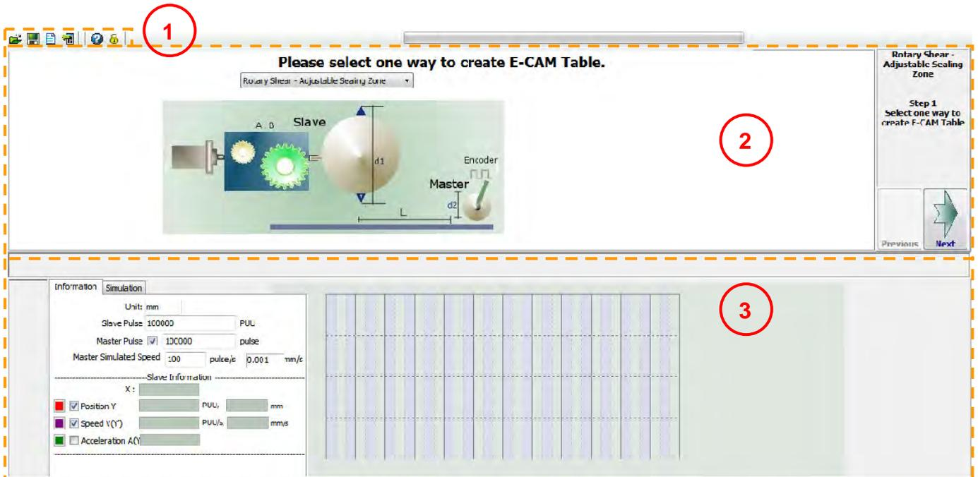
1. Toolbar: Open the E-Cam file or save the programmed E-Cam application.
