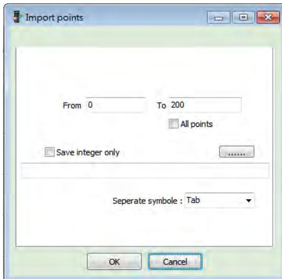
**[Import points]** Load in the first section, which has 200 parts. Its range is between 0 and 200. Then, load in the second one, which is from 200 to 400. The end position of the first section, 200 should be overlapped with the start position of the second section, 200.
