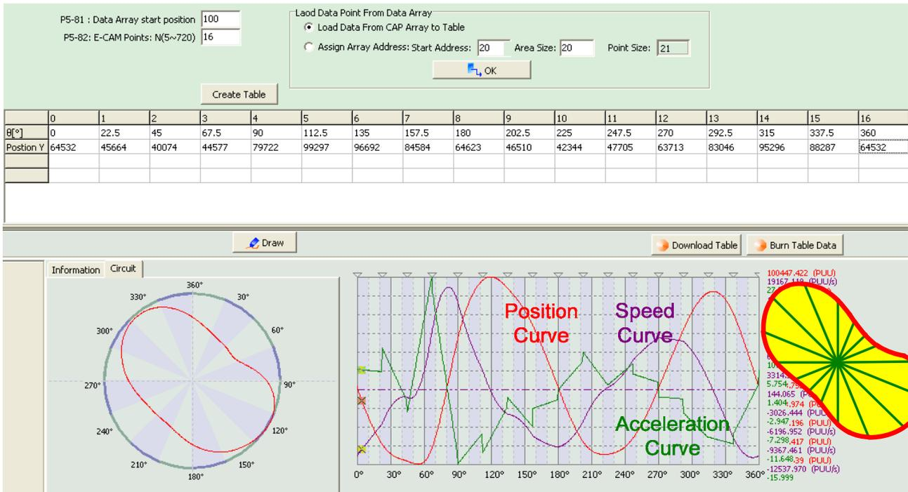
From the above figure, you may find that the E-Cam curve simulated by software is slightly different from the actual one which is marked on the right. It is because the above E-Cam curve is drew by 16 sampling points.
