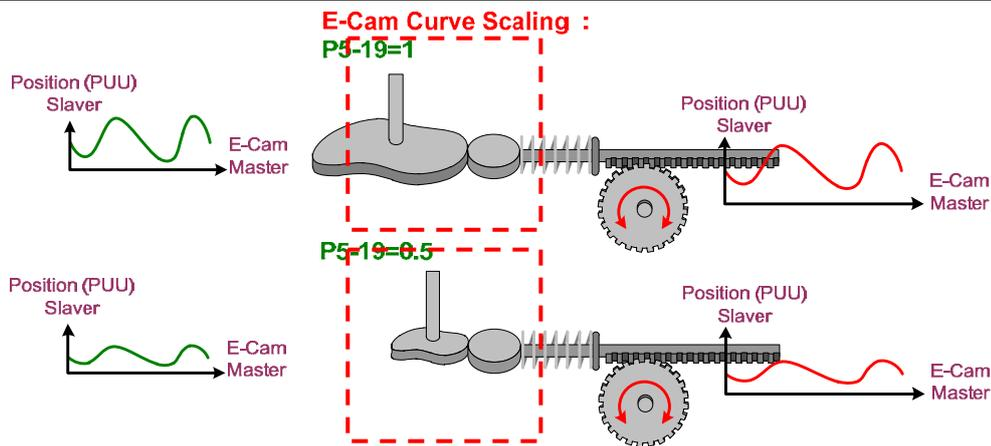
Effect brought by P5-19 is the same as E-gear of slave axis, but only influences E-Cam system. See as above. If P5-19 is set to 0.5, E-Cam axis will only output half of the PUU number, which is the same when adjusting P1-44 and P1-45, but it will not affect the E-gear ratio.
