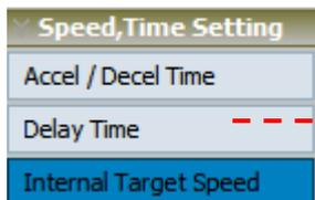
The unit of 16 sets of internal target speed is r/min. Its setting range is from 0.1 to 6000.0 r/min.
