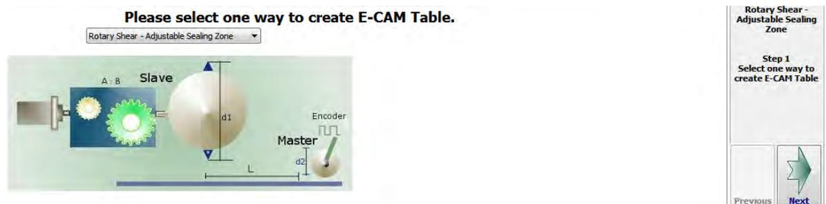
3. E-Cam sketch: According to the input pulse number of master and slave axis, the software will simulate the E-Cam curve.
