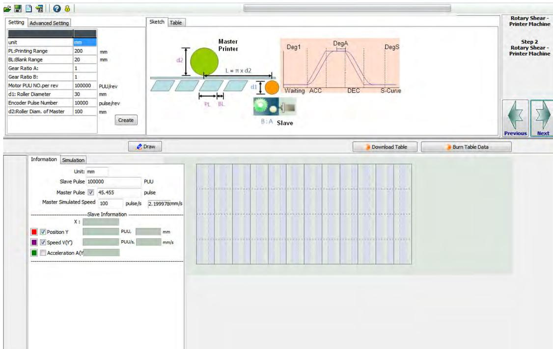
Parameter setting of mechanism is provided in “Setting”.
