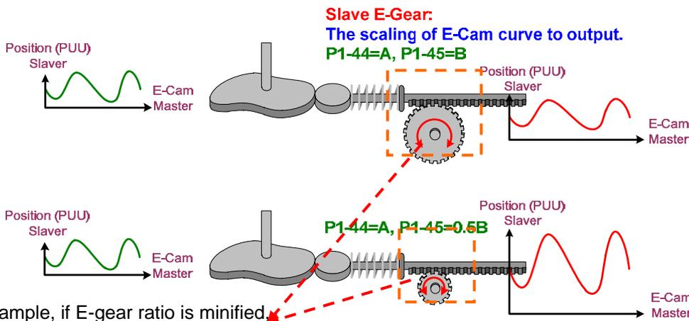
In this example, if E-gear ratio is minified, the position of slave axis will change. The system's E-gear ratio and the moving distance will be changed.
