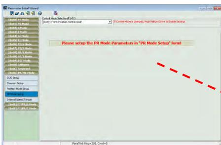
The prompting message in main screen: Setup the PR Mode in "PR Mode Setup
