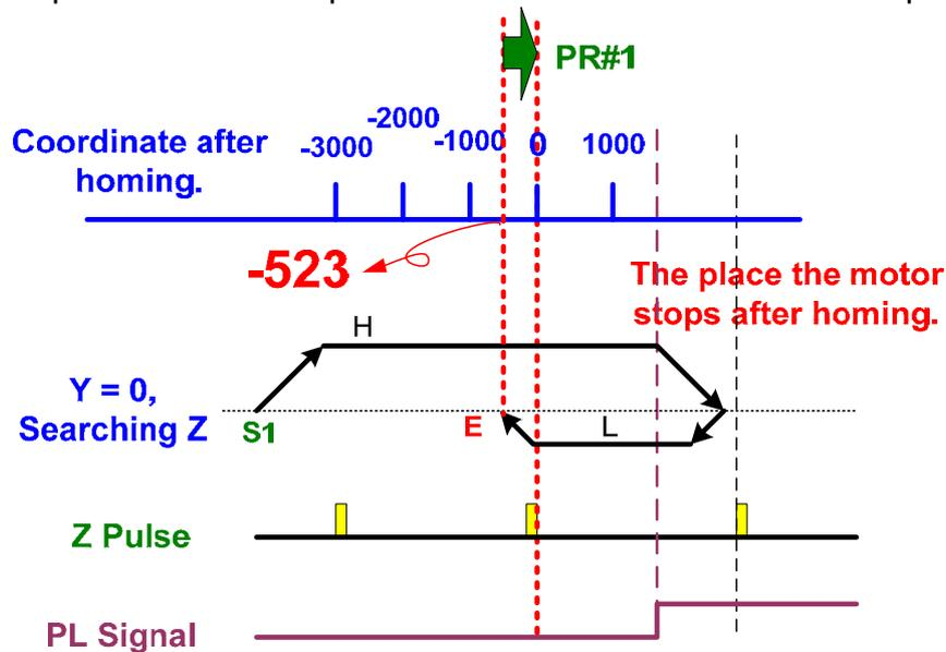
Through the software setting, users can command the motor returning to the origin point (absolute position 0). The first step is to specify one PR path.
