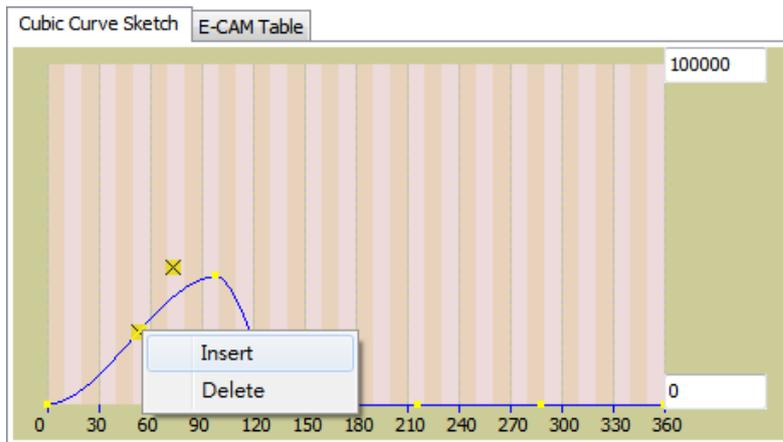
Select "Insert" and the software will add one point around the curve. Since both position and degree of this new point are 0, users have to manually enter these two values and re-program the curve type to create new points.
