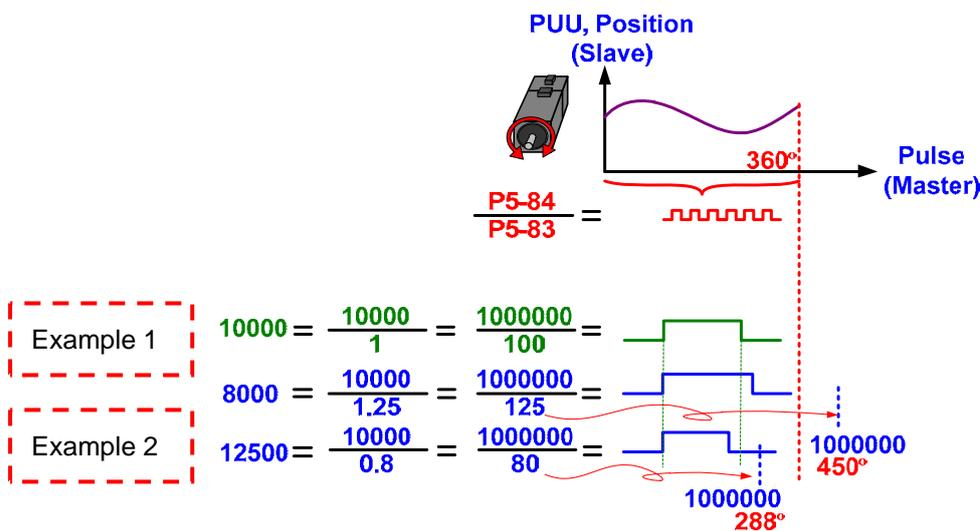
E-gear ratio of master axis changes the resolution of pulse command. P5-83 can be used for adjustment when it is engaged.
