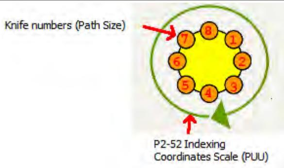
In first step, specify knife number and indexing coordinates scale (PUU). These two values relate to the coordinates (motor’s rotating angle) of each index point. For example, if indexing coordinates scale is set to 100,000PUU and knife number (path size) is 10, path of each index will be:  $\frac{100,000}{10} \equiv 10,000$  PUU
