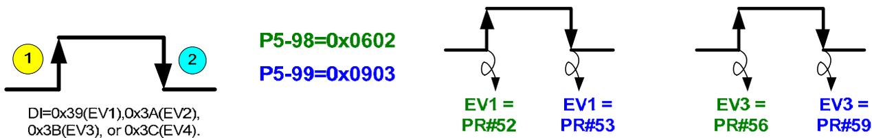
However, if we use drop-down menu of the software to setup, users only need to specify the PR of EV1 and EV3 and to complete the setting of DI (digital input) in **Parameter Initial Wizard**.
