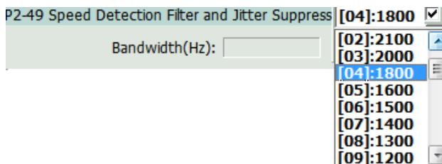
Following is the diagram of speed control: P2-49, low-pass filter, is used to process the feedback signal of encoder, which could reduce the interference and the error occurrence caused by speed control loop. Its setting value is from 100 to 2500 Hz.
