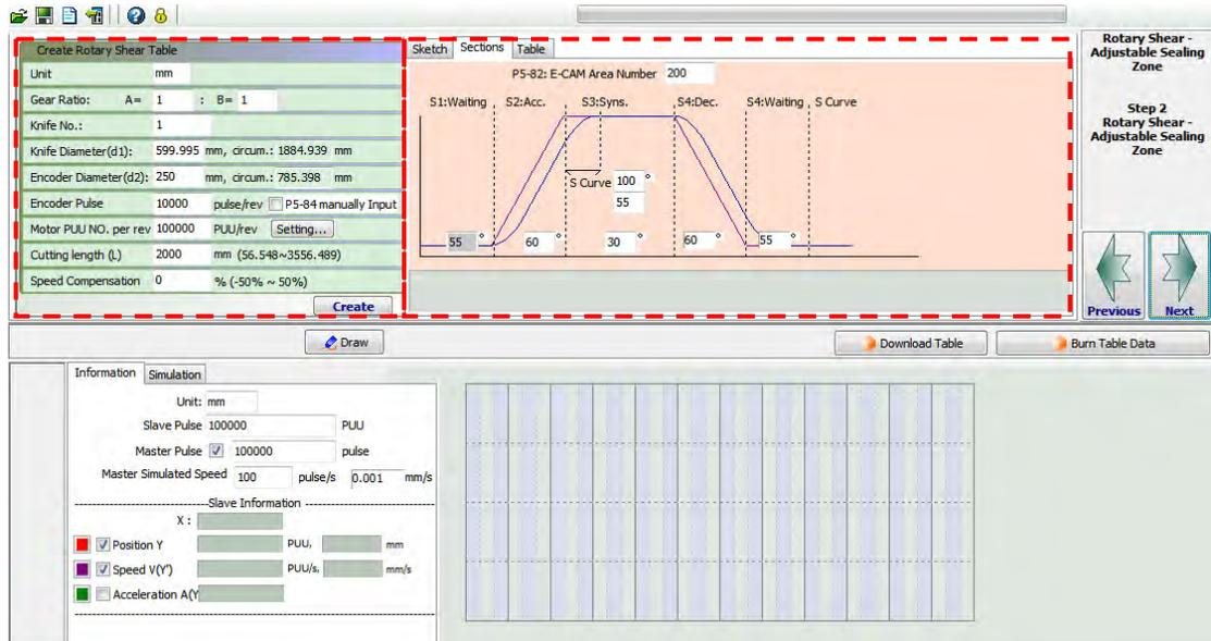
**Step 1:** Setup E-Cam area number. It is suggested to set the value to 72 to can bring the best curve resolution.
