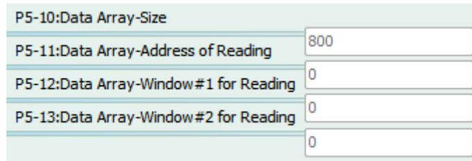
These four parameters cannot be modified in software. Users can only access their status via . If desire to read the value of data array so as to make sure the previous written content is correct, specify the start address to P5-11 through MODBUS communication command 0x06 (write one data). The issued command is showed as below:
