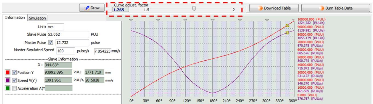
Confirm the diagram is correct. Then, users can download the table into the servo drive. If desire to keep the curve inside the servo drive when power off, click
