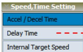
The unit of 16 sets of acceleration/deceleration time is ms. Its setting range is from 1 to 65,500ms.
