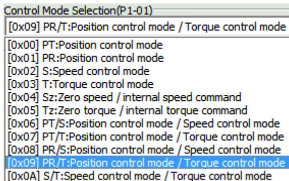
Step 2: Select Position control mode / Torque control mode, the setting block on the left will show as below:
