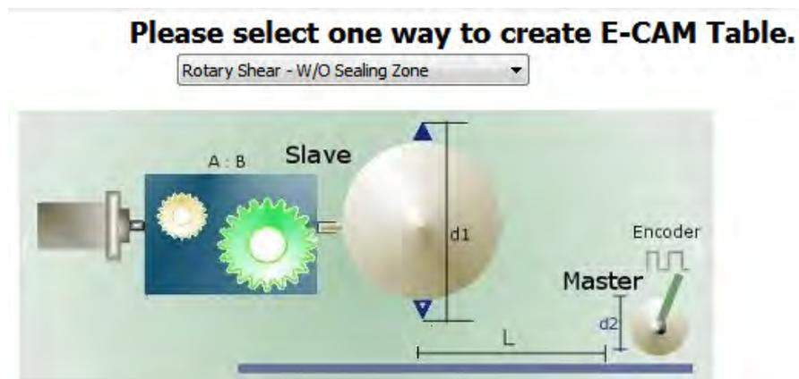
According to the above mentioned rotary shear curves, it provides three options for users:
