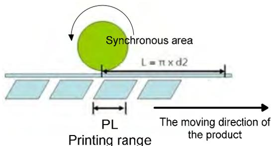
$\text{deg\_sync (Degree of synchronous area)} = PL / L \times 360^\circ$ . This formula can help to calculate the degree of synchronous area.
