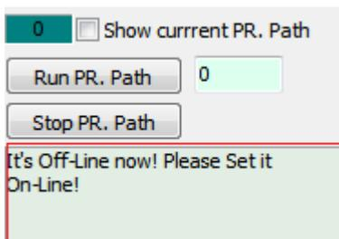
Check  Show current PR. Path when communication is OK, the status light will turn light green. Then, click “Run PR. Path”.
