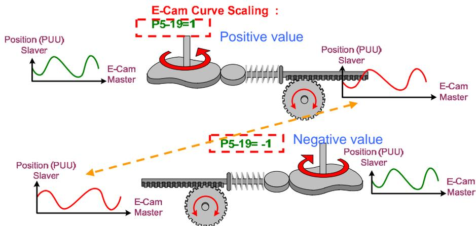
The value of P5-19 can be changed anytime. However, the change takes effect only when E-Cam is re-engaged (= leaves S1 status and back again). The change takes effect immediately in firmware version V1.038 sub48 (or later version).
