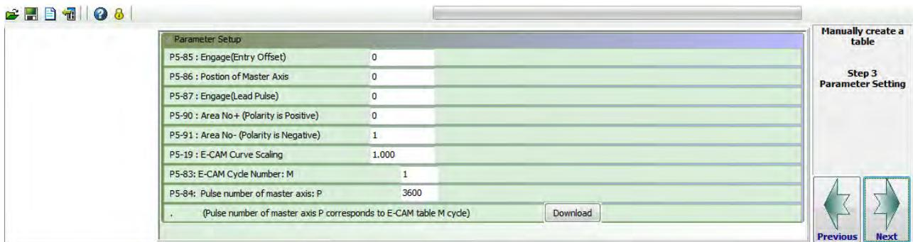
In this step, users can setup the following parameters according to the actual situation.
