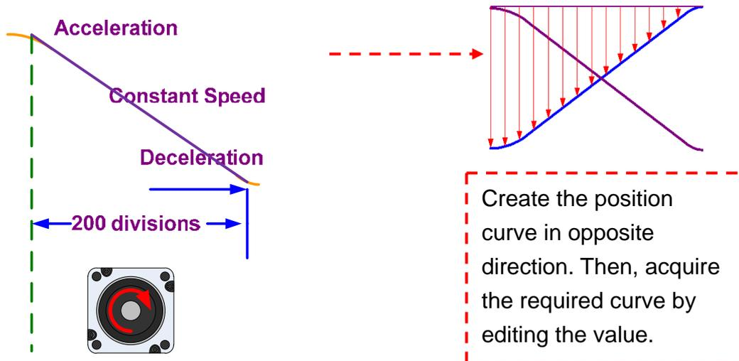
First, create the curve in opposite direction. 200 parts are in total. Then, enter the value according to the proportion of each area to acquire the curve in forward direction.
