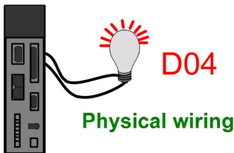
4. Software: Read the output signal from digital IO panel
