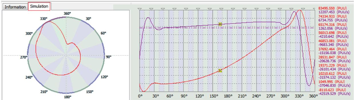
**Step 4:** Make sure the E-Cam curve is correct. Users can also use “Information” to simulate the master axis.
