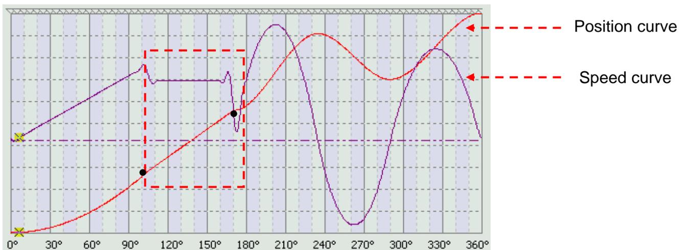
Assume the user needs to insert or delete points, users can directly edit on simulated curve by right clicking the mouse.
