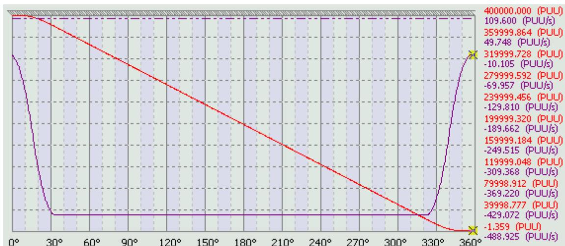
**Export the second section:** Right click the mouse at any column of the E-Cam table. Select “Export points”. Since there are 200 parts in this section, users should fill in values between 0 and 200. Then, save the data of the table.
