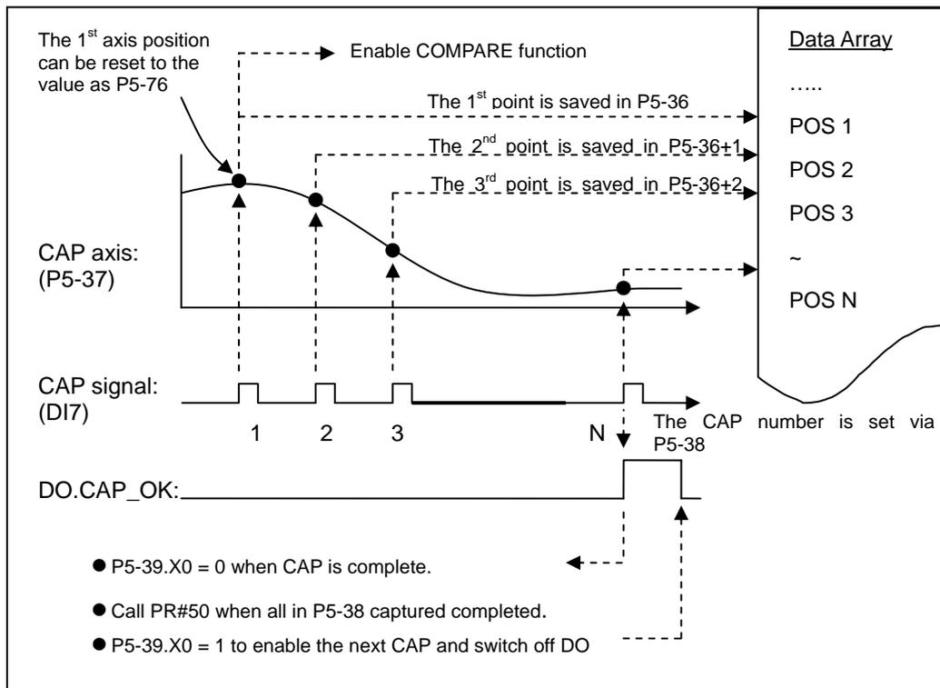
The concept of COMPARE is to compare the instant position of motion axis with the value which is saved in data array. Then output DO4 after the COMPARE condition is established for motion control. Since COMPARE is finished by hardware, there is no problem of software delay. It also can accurately compare the high-speed motion axis. The COMPARE features provided by ASDA-A2 servo drive is as follows.
