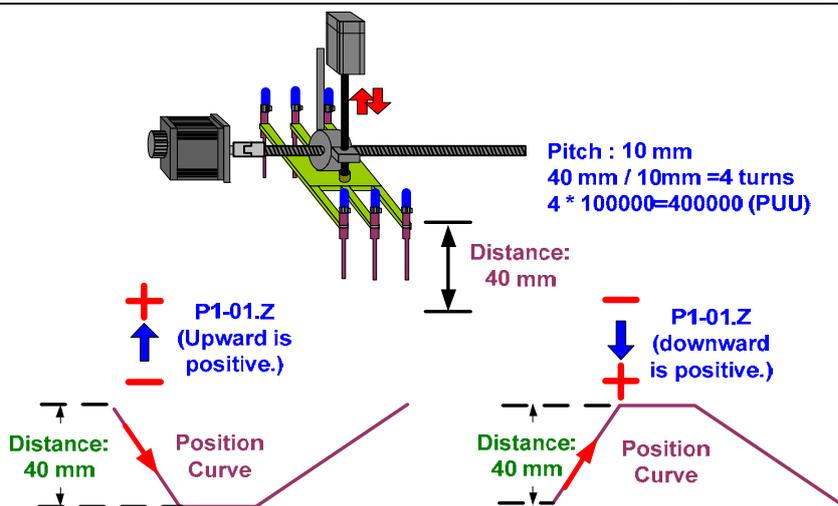
Before setting up forward and reverse curve, it is important to know that P5-18: Axis Position-Pulse Command (CN1); P5-86: E-CAM: Master Axis Position. When both pulse counts and feedback pulse counts increase at forward direction, the motor is defined to run at forward direction.
