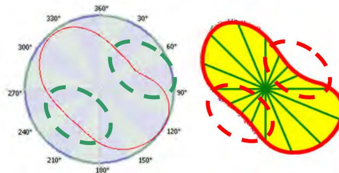
Actually, the built-in E-Cam in ASDA-A2 can be divided into 720 parts (721 points). The minimum degree of each part in one cycle (360°) is 0.5°.
