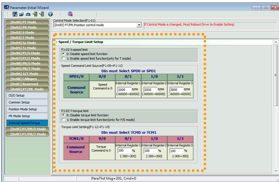
**[0x0E] PT/PR/S : Multi Control Mode (Position and Speed Mode)**
