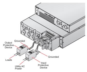
(Figure 7-1: Wiring Diagram)
