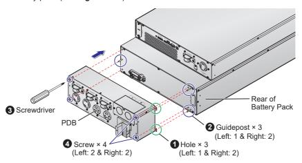
(Figure 6-12: Assemble the PDB)
