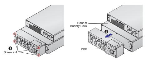
(Figure 6-11: Disassemble the PDB)
