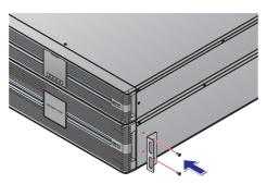
(Figure 6-1: UPS Bracket Ear Installation)
