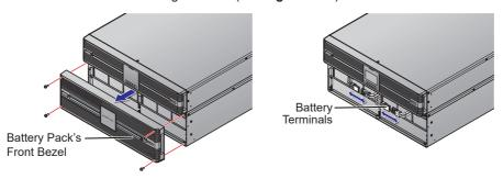
(Figure 6-10: Disconnect the Battery Power)
