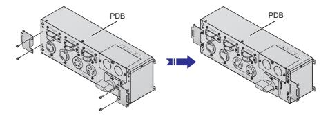
Attach the provided M5 nuts to the rack. Use the provided M5 screws to firmly install the PDB on the rack. Ensure that the screws are tightly fixed.
