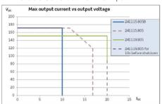
Figure 4 Output I/V diagram for 24111x.805
