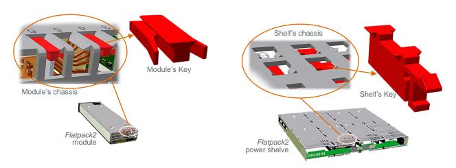
Figure 6 Keying scheme for Flatpack2 modules and power shelves (keys are black)
