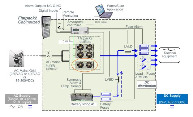
Figure 1 Typical Flatpack2 PS system for DC power supply of telecom equipment
