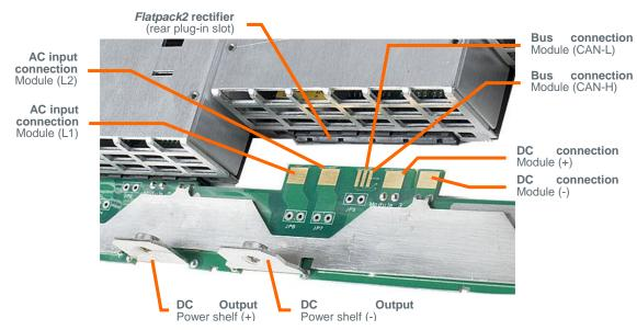
Figure 7 Flatpack2 module's rear plug-in connections to power shelf's back wiring card
