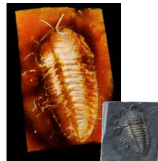
▲ DELab \mu CT-100X Trilobite fossil 40 kVp, 0.5 mmAl Resolution: 3 \mu m
