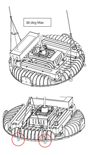
Connect power cable conductors as follows: Green/Yellow wire connects to Safety Ground. Blue wire connects to Neutral. Brow wire connects to Live.
