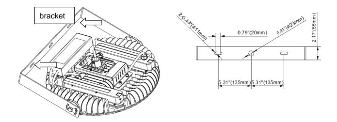
2. Loosen the M10 and M4 screw, and tilt the luminaire to the determined direction. If determined, fixed the Screw.
