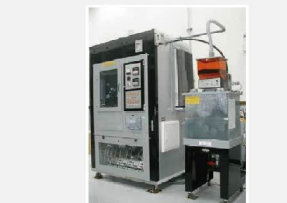
Flow Gas Corrosion
