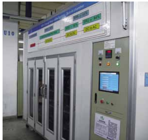
Delta's Energy Recycling System (ERS) is now able to recycle up to 95% of the electricity used during burn-in testing.
