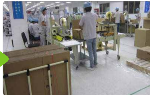
After: Automatic strapping machines. The packing process is more efficient and requires two fewer workers.
