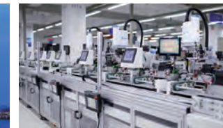
SCARA Robot with machine vision system for a function test of AC motor drives in China
