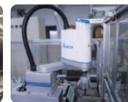
SCAR robot solution with machine vision system for function testing of AC motor drives in China
