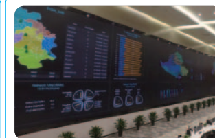
The world's largest video wall with 324 LED DLP 80' cubes and DVCS system in China
