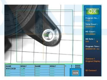
The picture below shows the DMV detecting a cutting-edge of the screw thread lower than the standard set value and confirms if the tapping is unsuccessful.
