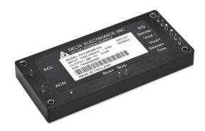
The PACSR series has two output power levels, 300W and 500W. It operates at universal AC input voltage from 85~264VAC, and has four output voltage of 12V, 24V, 28V, and 48V available with voltage trimming function. The standard features of PACSR series include over temperature protection, input under voltage protection, and output over current and over voltage protection.
