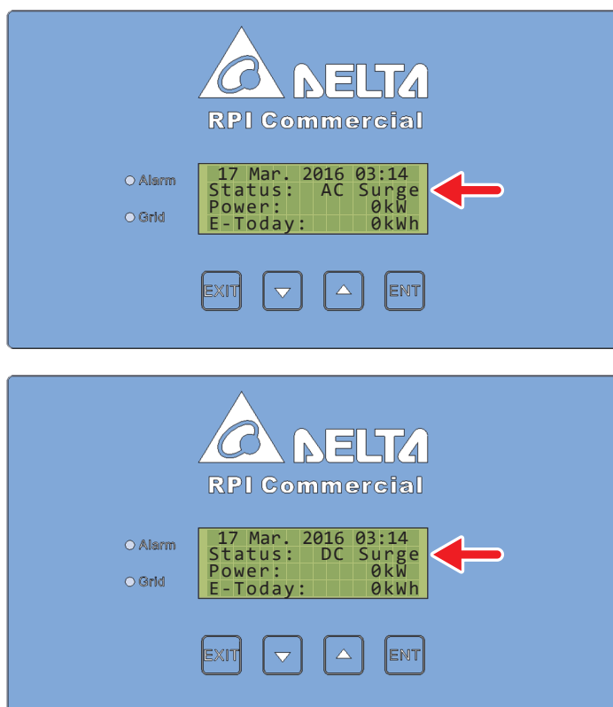
Figure 5-4: Display Indicating AC and DC SPD failure
