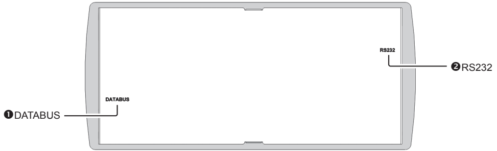
(Fig. 2-9: Back View of the Control Panel)
