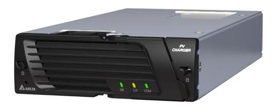
PVC 2500B RenE is the photovoltaic battery charger, and it can help convert the solar energy to -48V power system. PVC 2500B RenE can fit in standalone application and the hybrid power applications, such as genset supply, AC grid, wind energy and fuel cell supply. With the modularity, PVC 2500B RenE can be embed in the power system really easy, not only about the installation, but also the commissioning and the maintenance.
