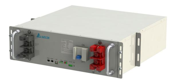
This new Delta 51.2 V battery pack is designed with a 100 Ah capacity battery cell of lithium-ion iron phosphate chemistry. It provides larger capacity in the compact size of a 19" rack-mounted 3U chassis. This pack has RS485 communication and a built-in BMS with automatic protection and cell balancing to offer safe and highly efficient operation to customers.
