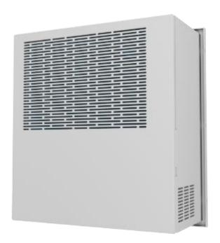
Delta TCAC-350 Series is the -48V DC input cooling system for telecommunication applications. Compact design to save the space to reduce cabinet size. DC inverter compressor for energy saving. Two mode standalone operation or integrated with Delta Telecom system controller. And Environment Friendly R134a refrigerant and full RoHS compliant design.
