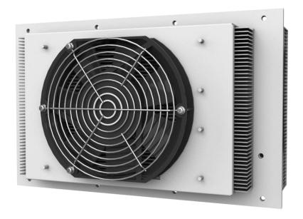
Delta TCTC-160 Series thermoelectric cooler (TEC) is designed for air to air heat dissipation module in the cabinet. The internal and external air circulation loops of the TEC module are separated to prevent the ingress of dust, humidity, and salt.
