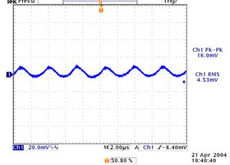
Figure 7: Output ripple & noise at 3.3Vin, 2.5V/10A out
