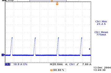
Figure 27: Output short circuit current 5Vin, 0.75Vout
