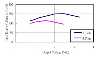
**Figure 33:** Input voltage ripple for various output models, IO = 10 A (CIN = 4×100 µF tantalum // 2×47 µF ceramic)
