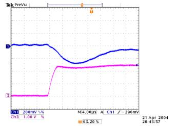
Figure 24: Typical transient response to step load change at 2.5A/µS from 50% to 100% of Io, max at 3.3Vin, 2.5Vout (Cout =1uF ceramic, 10µF tantalum)
