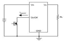
Figure 34: Positive remote On/Off implementation
