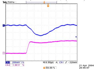
Figure 26: Typical transient response to step load change at 2.5A/ $\!\mu S$  from 50% to 100% of Io, max at 3.3Vin, 1.8Vout (Cout = 1uF ceramic, 10µF tantalum)
