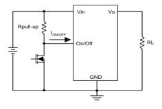
Figure 35: Negative remote On/Off implementation
