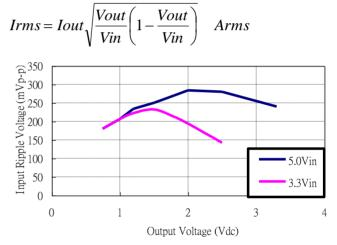
**Figure 32:** Input voltage ripple for various output models, IO = 10 A (CIN = 2×100  $\mu$ F tantalum // 47  $\mu$ F ceramic)
