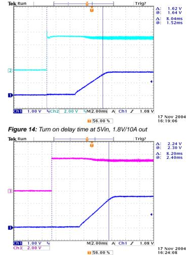
Figure 16: Turn on delay time at remote turn on 3.3Vin, 2.5V/16A
