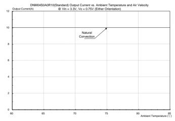
**Figure 48:** DNM04S0A0R10 (Standard) Output current vs. ambient temperature and air velocity @ Vin=3.3V, Vo=0.75V(Either Orientation)
