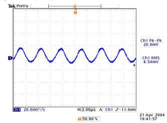
Figure 9: Output ripple & noise at 5Vin, 3.3V/10A out
