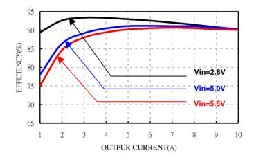
Figure 4: Converter efficiency vs. output current (1.5V out)
