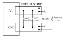
Note: Use a  $10\mu$ F tantalum and  $1\mu$ F capacitor. Scope measurement should be made using a BNC cable.
