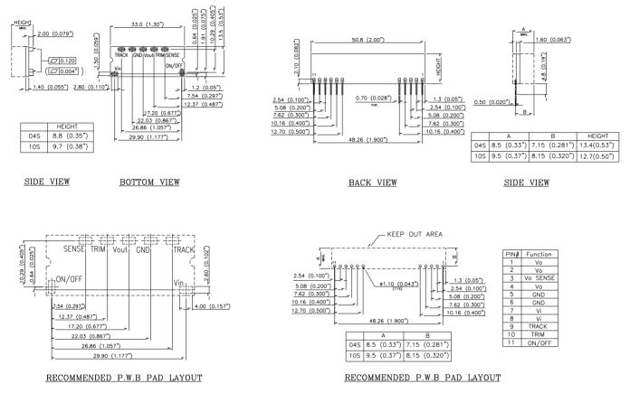
NOTES: DIMENSIONS ARE IN MILLIMETERS AND (INCHES) TOLERANCES: X.Xmm±0.5mm(X.XX in.±0.02 in.) X.XXmm±0.25mm(X.XXX in.±0.010 in.)
