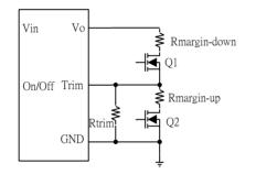
Figure 39: Circuit configuration for output voltage margining
