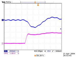
**Figure 22:** Typical transient response to step load change at 2.5A/µS from 50% to 100% of lo, max at 5Vin, 1.8Vout (Cout = 1uF ceramic, 10µF tantalum)
