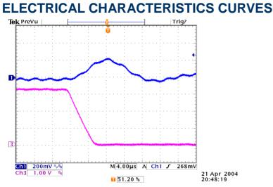
**Figure 19:** Typical transient response to step load change at 2.5A/µS from 100% to 50% of lo, max at 5Vin, 3.3Vout (Cout = 1uF ceramic, 10µF tantalum)
