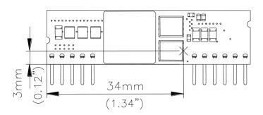
Figure 44: Temperature measurement location \* The allowed maximum hot spot temperature is defined at 125  ${\rm \mathcal{C}}$
