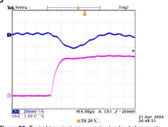
**Figure 20:** Typical transient response to step load change at 2.5A/μS from 50% to 100% of lo, max at 5Vin, 3.3Vout (Cout =1uF ceramic, 10μF tantalum)
