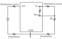
Figure 36: Effective circuit configuration for remote sense operation
