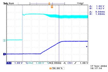
Figure 12: Turn on delay time at 3.3Vin, 1.8V/10A out
