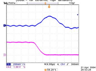
**Figure 21:** Typical transient response to step load change at 2.5A/μS from 100% to 50% of Io, max at 5Vin, 1.8Vout (Cout =1uF ceramic, 10μF tantalum)
