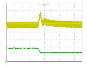
**Figure 8:** Output voltage response to step-change in load current (75%-50% of Io, max; di/dt =  $0.1A/\mu$ s, Vin=54V). Load cap:220 $\mu$ F, electrolytic capacitor ;  $10\mu$ F, tantalum capacitor and  $1\mu$ F ceramic capacitor. Top Trace: Vout (200mV/div, 200us/div); Bottom Trace: Io (10A/div, 200us/div). Scope measurement should be made using a BNC cable (length shorter than 20 inches). Position the load between 51 mm to 76 mm (2 inches to 3 inches) from the module..
