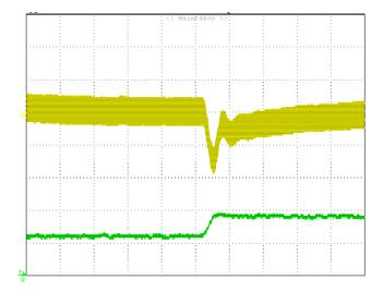
**Figure 9:** Output voltage response to step-change in load current (50%-75% of Io, max; di/dt =  $0.1A/\mu$ s, Vin=54V). Load cap: 220 $\mu$ F, electrolytic capacitor ;10 $\mu$ F, tantalum capacitor and 1 $\mu$ F ceramic capacitor. Top Trace: Vout (200mV/div, 200us/div); Bottom Trace: Io (10A/div, 200us/div). Scope measurement should be made using a BNC cable (length shorter than 20 inches). Position the load between 51 mm to 76 mm (2 inches to 3 inches) from the module..
