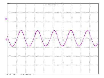
**Figure 14:** Output voltage ripple at nominal input voltage and rated load current (Io=25A)(50 mV/div, 2us/div) Loadcapacitance:220uF(Electrolytic)+10uF(Tantalum)+1uF(Ce ramic) and min Co. Bandwidth: 20 MHz.
