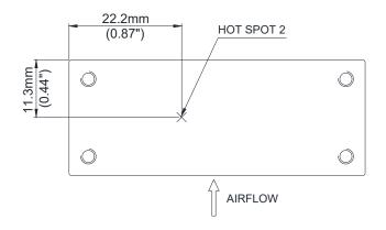
**Figure 24:** \* Hot spot 2 temperature measured point, the allowed maximum hot spot 2 temperature is defined at 101 C
