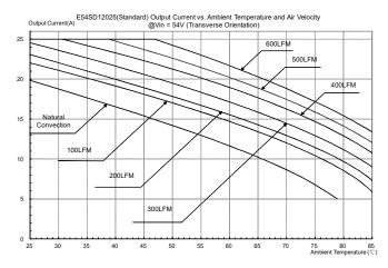
**Figure 23:** Output current vs. ambient temperature and air velocity @Vin=54V(Transverse Orientation, airflow from Vinto Vin+, without heat spreader)
