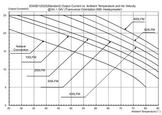
**Figure 26:** Output current vs. ambient temperature and air velocity @Vin=54V(Transverse Orientation, airflow from Vin-to Vin+, with heat spreader)
