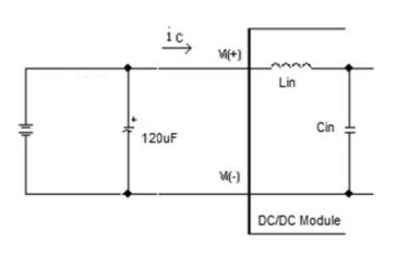
Figure 9: Test Setup Diagram for Input Ripple Current Note: Measured input ripple current with a simulated source, with 100 $\mu$ F AL cap and 20 $\mu$ F ceramic cap. Measure current as shown above.
