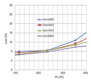
Figure 2: Loss vs. Output Power
