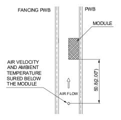
Note: Wind Tunnel Test Setup Figure Dimensions are in millimeters and (Incl
