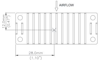
Figure 20: Hot spot 2 temperature measurement location The allowed maximum hot spot 1 temperature is defined at 110  $\mathcal{C}$ . The allowed maximum hot spot 2 temperature is defined at 105  $\mathcal{C}$ .
