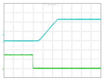
Figure 5: Remote On/Off (negative logic) at full load Vin=54V, I<sub>out</sub> =33.9A Time: 5ms/div. V<sub>out</sub> (top trace): 5V/div; V<sub>remote On/Off signal</sub> (bottom trace): 2V/div.
