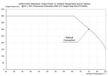
Figure 21: Output Power vs. Ambient Temperature and Air Velocity @Vin = 54V (Transverse Orientation, Airflow from Vin+ to Vin-, With 0.5" Height Heat Spreader ETL050A)
