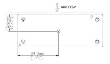
Figure 18: Hot spot 1 temperature measurement location
