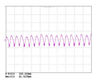
**Figure 10: Input Ripple Current**, i<sub>c</sub>, at max output current and nominal input voltage with 100 $\mu$ F AL cap and 20 $\mu$ F ceramic cap. (200 mA/div, 2us/div).
