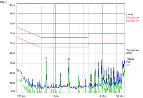
Figure 13-2: Test Result of EMC(Vin=54V, Io=33.9A).
