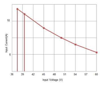
Figure 3: Full Load Input Characteristics
