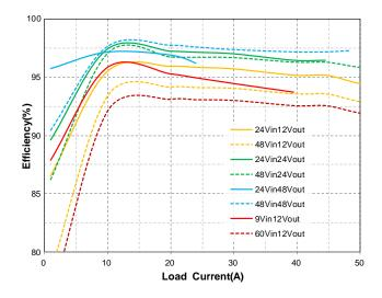
Figure 1: Efficiency vs. Load Current at Ta=25°C
