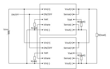
Figure 16: Parallel and current sharing configuration
