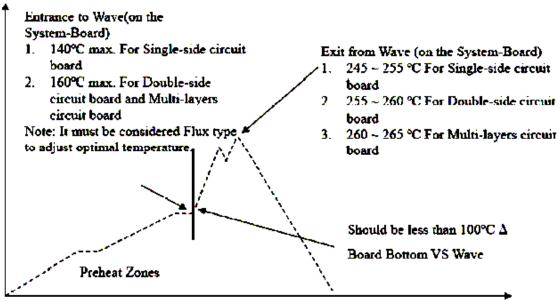
Recommended Temperature Profile for Lead-free Wave Soldering
