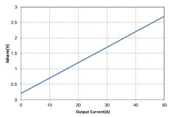
Figure 8: Ishare/Imon pin voltage vs. output load current.
