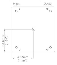
Figure 18: \* Hot spot's location on the base plate.
