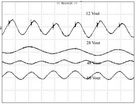
**Figure 12: Input Terminal Ripple Current**, i<sub>c</sub>, at max output current and nominal input voltage(28V) with 12µH source impedance and 33µF electrolytic capacitor (50 mA/div, 2us/div).
