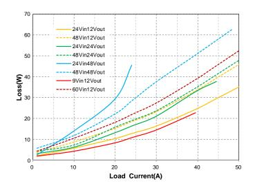
Figure 2: Loss vs. Output Power at Ta=25°C
