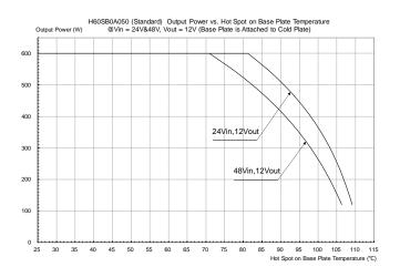
**Figure 19:** Output power vs. Base plate temperature @Vin=24V&48V, Vout=12V (Base plate is attached to cold plate)
