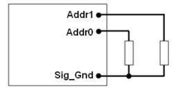
Corresponded to each octal digit, the requested resistor values are shown in below, and +/-1% resistors accuracy can be accepted. If there are any resistances exceeding the requested range, address 127 will be return. 0-12 and 40, 44, 45, and 55 in decimal address can't be used, since they are reserved according to the SMBus specifications, and which will also return address 127. The address resistance will be considered as 200k if resistor ≥200k.
