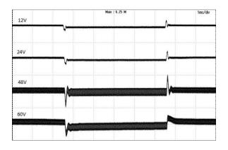
**Figure 9: Transient Response** (28Vin, di/dt=0.1A/Us, from top trace to bottom trace 12Vout, 25A-37.5A-25A; 24Vout, 25A-37.5A-25A; 48Vout, 12A-18A-12A; 60Vout, 5A-7.5A-5A. 2V/div, 1ms/div; Cout is 100uF.
