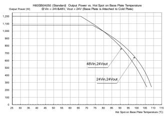
**Figure 20:** Output power vs. Base plate temperature @Vin=24V&48V, Vout=24V (Base plate is attached to cold plate)
